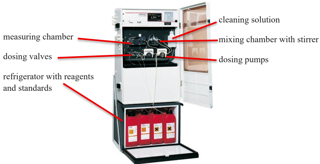
Fig. 18: Analyser for photometric real-time measurement of ammonium (Hach, 2026f) (used by permission of Hach Company).
