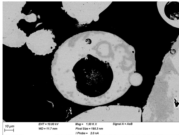
Figure 5.9: Example of unmelted powder particle containing one large and one small pore, as well as crystals (darker regions). This particle was found in a large hole within a built sample.
