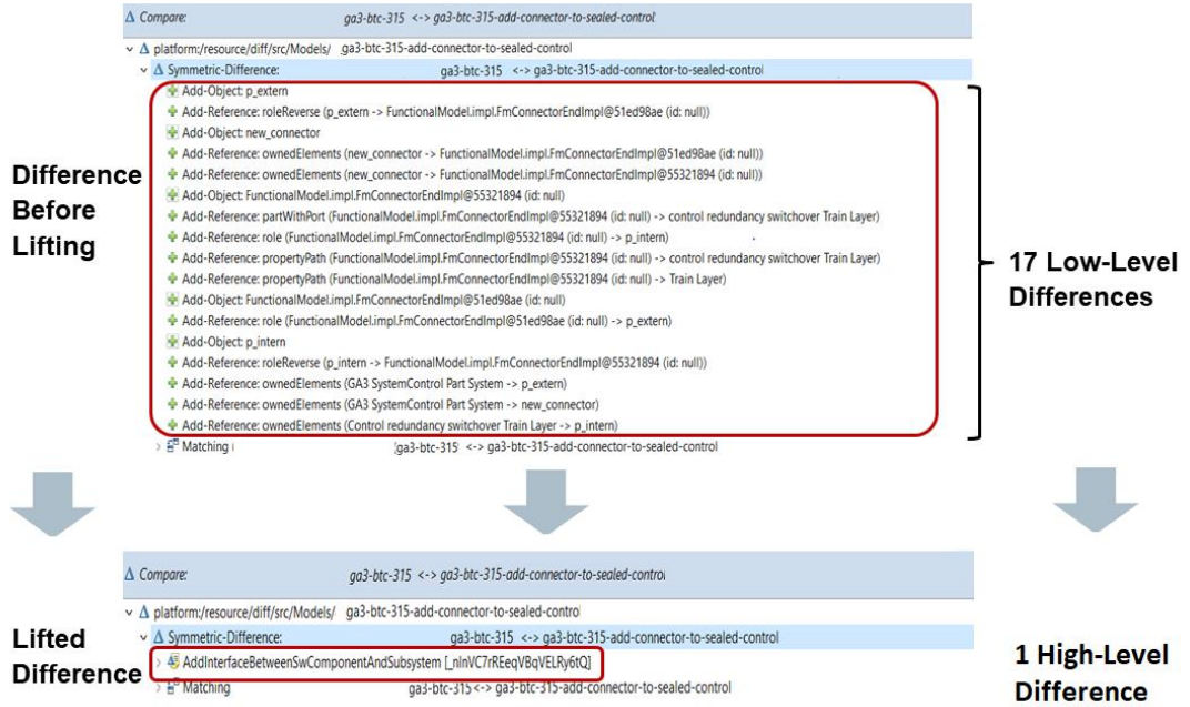
Figure 4.6: Results of the semantic lifting of a connector that is added between a component and a subsystem.
