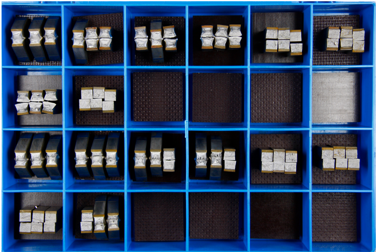
Fig. 2. Industrial recording to document the fracture behavior of the different test conditions. One compartment within the box represents a specific test configuration – each tested using 3 samples.
