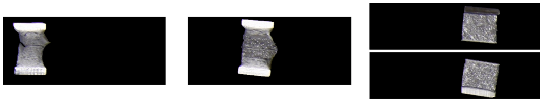
Fig. 9. Charpy V-notch specimen using prediction masks to extract the 3 samples from the sample bundle of Fig. 4.
