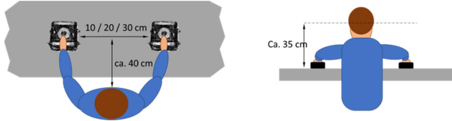
Figure 3.40: User test setup for local assignability tests with two units. User position and different locations of the demonstrators ([216]).
