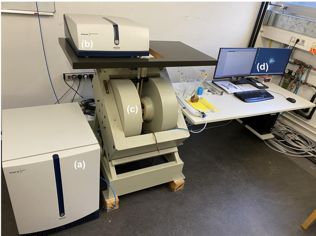
**Fig. 2.1** Experimental setup of the continuous wave (CW) EMX X-band ESR spectrometer with console (a), microwave bridge (b), Helmholtz coils (c) and data acquisition software at a computer (d). [96]
