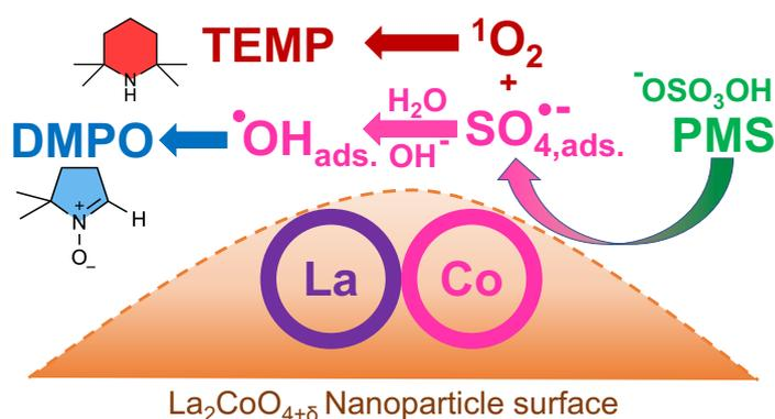
**Fig. 4.4** Reaction pathway of the activation of peroxymonosulfate (PMS) via  $\text{La}_2\text{CoO}_{4+\delta}$  nanoparticles. In the beginning, sulfate radicals and singlet oxygen are formed with subsequent formation of hydroxide radicals in aqueous environment. TEMP is used as radical scavenger for singlet oxygen, while DMPO is used as radical scavenger for  $\text{OH}^-$ - and  $\text{SO}_4^-$ -radicals.
