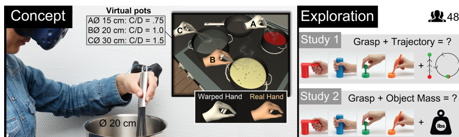
Figure 5.1: Lisa moves a proxy whisk inside a proxy pot (left). Visuo-Haptic Rotation works by offsetting the virtual hand/tool from the real hand/tool. We can simulate virtual pots of different sizes, which provide realistic haptic sensations when stirring. Our studies investigate the extent to which we can use such illusions by exploring the potential effects of grasp, movement trajectory and object mass on the offset which can be introduced while remaining unnoticed by a user.
