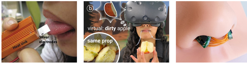
Figure 2.5: Left: Thermal device that actuates the taste receptors of the tongue, creating the sensation of sweetness. (Source: extracted from Karunanayaka et al. [176] ©2018). Middle: Chemical modulators can alter users' taste perception. (Source: extracted from Brooks et al. [43] ©2023). Right: Electrical stimulation device that produces stereo-smell. (Source: extracted and cropped from Brooks et al. [44] ©2021).
