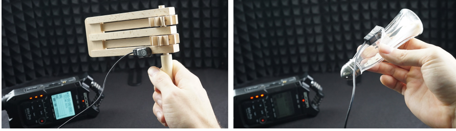
Figure 3.13: Recording vibrations from real-world object interactions using a condenser vibration pickup microphone.
