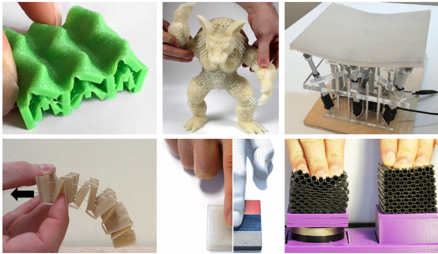
Figure 2.23: Top left: 3D-printed metamaterial textures. (Source: extracted and cropped from Ion et al. [159]; ©2018). Top middle: 3D-printed microstructures to control elasticity. (Source: extracted and cropped from Schumacher et al. [297]; ©2015). Top right: A mechatronic shape display based on auxetic materials. (Source: extracted and cropped from Steed et al. [320]; under CC BY 4.0). Bottom left: Strings to compress metamaterials, creating shape-change. (Source: extracted and cropped from Neville et al. [252]; under CC BY 4.0). Bottom middle: 3D-printed hairs with visual texture overlays to create combined visuo-haptic perception. (Source: extracted and cropped from Degraen et al. [69]; ©2019). Bottom right: 3D printing objects with varying deformation properties. (Source: extracted and cropped from Piovarči et al. [271]; ©2016).
