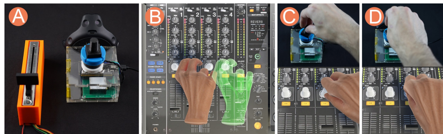
Figure 4.9: (A) displaying our knob proxy next to our slider proxy developed in the section below. (B) shows a user's hand is redirected. (C) indicates the start position, while (D) shows the position of the hand after rotation in the real and virtual world.
