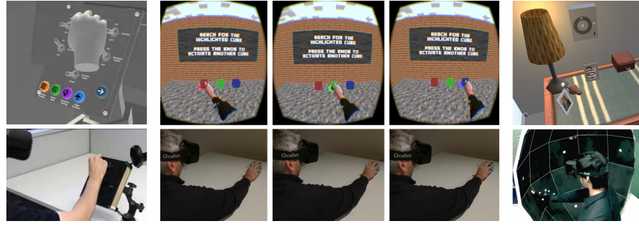
Figure 2.27: Examples of haptic retargeting. Left: Virtual sliders, buttons and knobs embodied by a proxy. (Source: extracted and cropped from accompanying paper video by Matthews et al. [237]; ©2023). Middle: Single proxy cube provides touch feedback for multiple virtual cubes. (Source: extracted and cropped from Azmandian et al. [17]; ©2016 ACM). Right: Sparse Haptic Proxy in combination with HR renders touch feedback. (Source: extracted and cropped from Cheng et al. [52]; ©2017).
