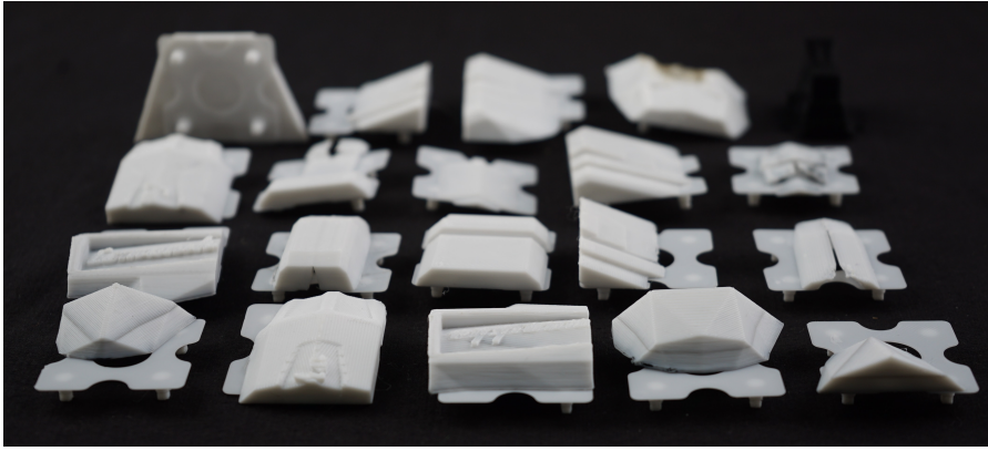
Figure 3.5: 3D-printed ShapePlates of the power drill that can be attached to the low fidelity power drill to increase shape resolution.
