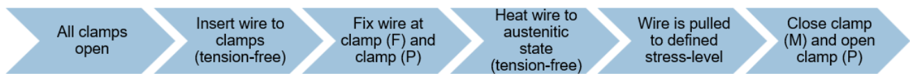
Figure 5. Flowchart of the installation procedure of a SMA wire specimen in the test rig.
