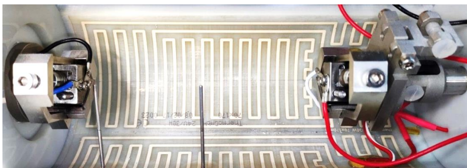
Figure 3. Picture of the inside of the chamber with heating foil, both wire clamps with a SMA wire sample installed, electrical wiring and PT100 sensor tips.
