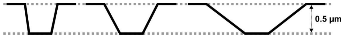
Figure 22. Schematic illustration of experimental design to probe hypothesis A. Friction testing will be conducted on 3 laser structures (CNT-coated) with identical structural depths but different slope angles.
