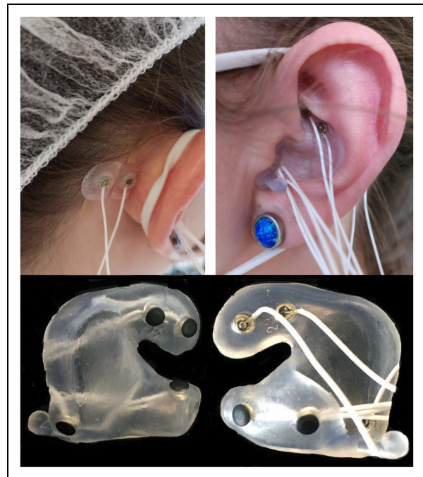
Figure 2. Top: Electrodes attached to the postauricular muscle (PAM), as well as an inserted earpiece including the electrodes. Bottom: Close-up of an earpiece with inserted electrodes. Two electrodes are located at the upper part of the concha, while the other electrodes are placed inside the ear canal or at the tragus/anti-tragus.
