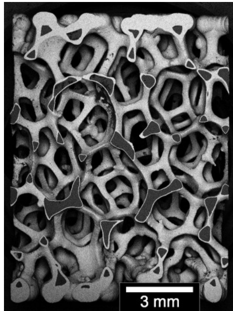
Figure 1.1: Coated foam with significant coating thickness inhomogeneities, Bouwhuis et al. [25]
