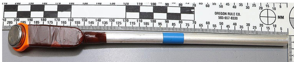
Fig. 1 DS1922L data logger after removal of protective layers. Note blue marking at 120 mm distance to tip of logger assembly
