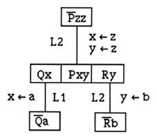
Link L1 ist compatible with L2 and L1 is compatible with L3, but L1, L2, L3 are not simultaneously compatible and L1 can therefore be deleted.
