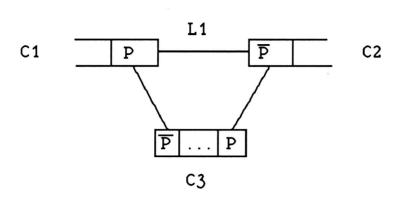
If the link L1 is missing, possible deduction steps can be lost by the deletion of the tautology C3. The existence of the link L1 is here termed as "link condition". For the other reduction rules subsumption, replacement factoring, replacement resolution similar link conditions exist. These link conditions make several additional checks necessary:
