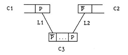
In this case the link condition is not fulfilled and the tautology C3 cannot be deleted. Deleting L1 or L2 causes the link condition to become superfluous and C3 can be deleted.
