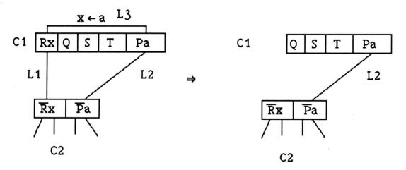
The link L3 is inserted by the two-rule-algorithm and makes a replacement factoring possible.
