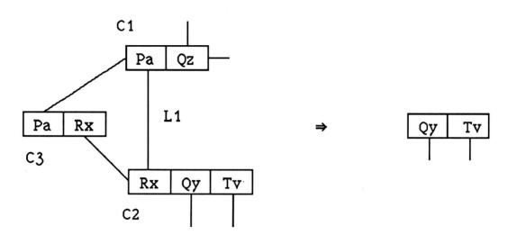
L1 is inserted by the two-rule-algorithm. The clause  $\langle Qy, Tv \rangle$  resulting by resolving upon link L1 would subsume C2. Therefore C2 can be replaced by  $\langle Qy, Tv \rangle$
