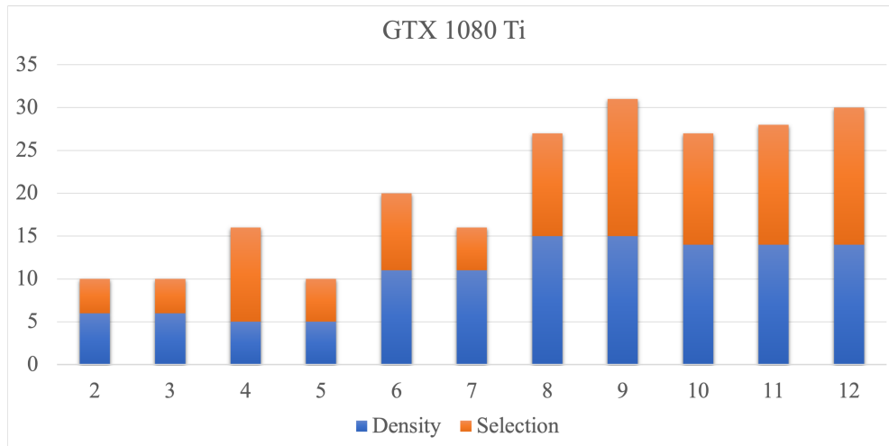
Figure 5.37: Runtime in milliseconds on the GTX 1080 Ti (smaller is better, based on performance numbers published in [KK18]). Blue : Density approximation. Orange : Selection process.
