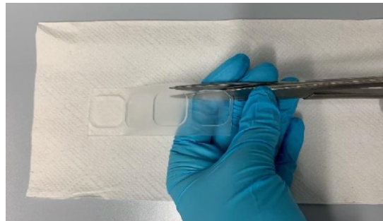
Supplementary Figure 9: Remove protruding PDMS that surrounds the entities with scissors.
