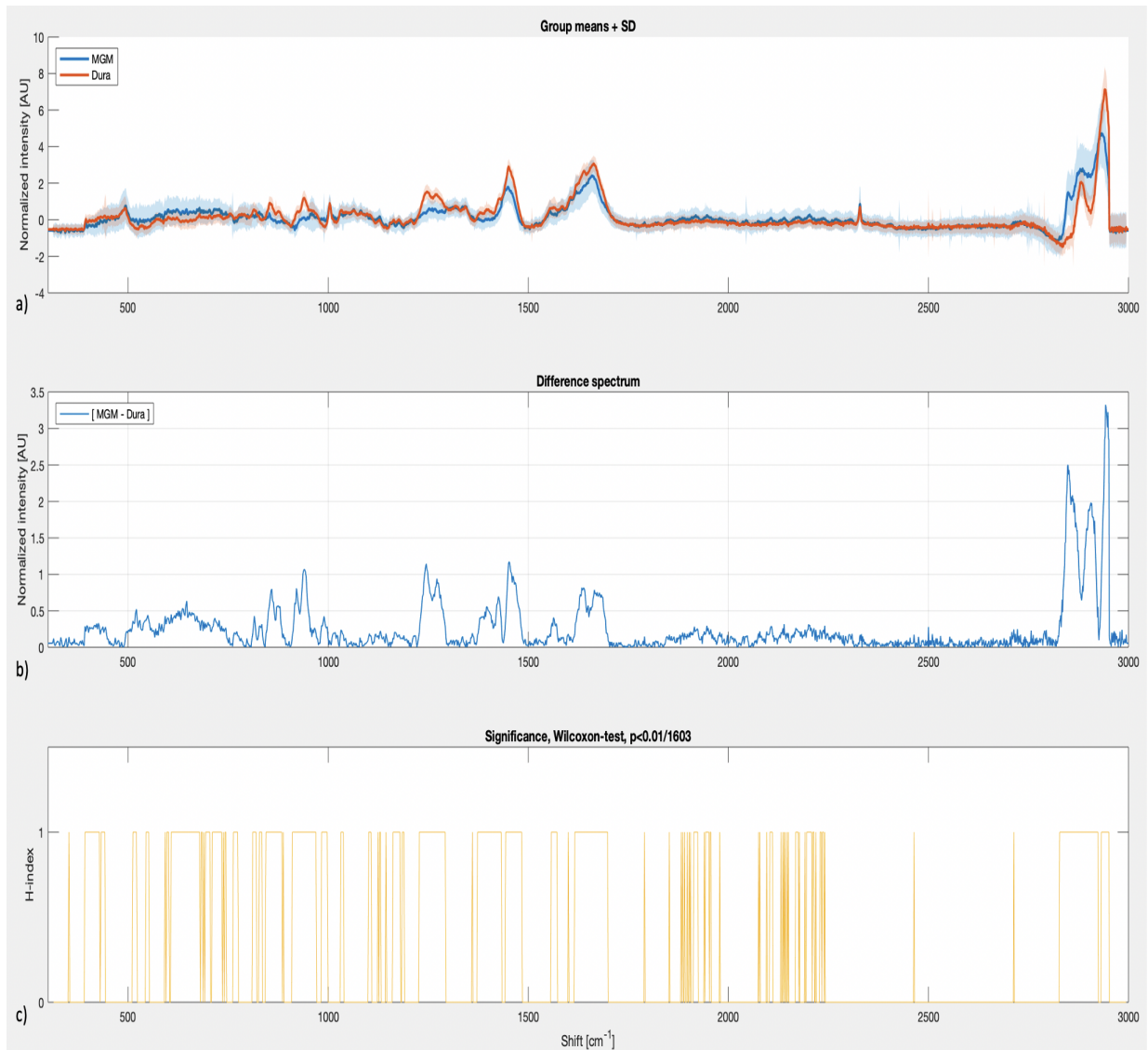
Figure20: (a) Average spectra with the individual standard deviations of meningioma and dura mater measurements. A spectral difference can be observed; (b) Subtraction of the mean dura mater spectrum from the mean meningioma spectrum; (c) Significance at each single Raman shift (0=null hypothesis, 1=alternative hypothesis) calculated using Wilcoxon-Mann-Whitney-U test, p-value is Bonferroni-corrected, resulting in p \leq 6 \times 10^{-6} . Multiple significant differences can be observed. Figure source: Jelke, Mirizzi et al. 2021; Scientific-reports 2021, "Reproduced with permission from Springer Nature" 75
