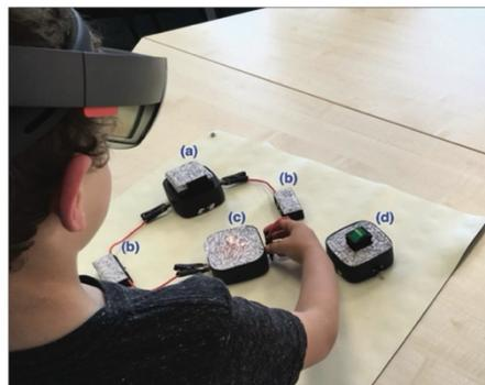
Fig. 1. A student building a circuit with the HoloLens setup using battery (a), cables (b), light bulb (c) and switch (d).
