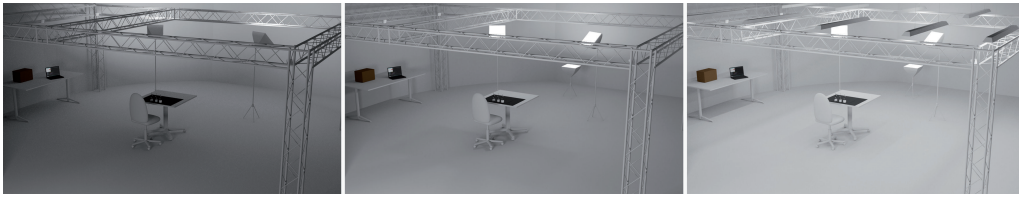
Figure 4.9: Illustrations of the laboratory setup in our three lighting conditions Dark, Medium and Bright (left to right). Studio lamps and lamps on the ceiling were used to adjust the environmental illuminance.
