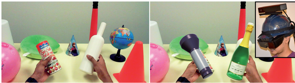
Figure 2.21: Virtually overlaid everyday proxy objects determined by the algorithm of Hettiarachchi and Wigdor [55] (right). Scene without overlays (left).
