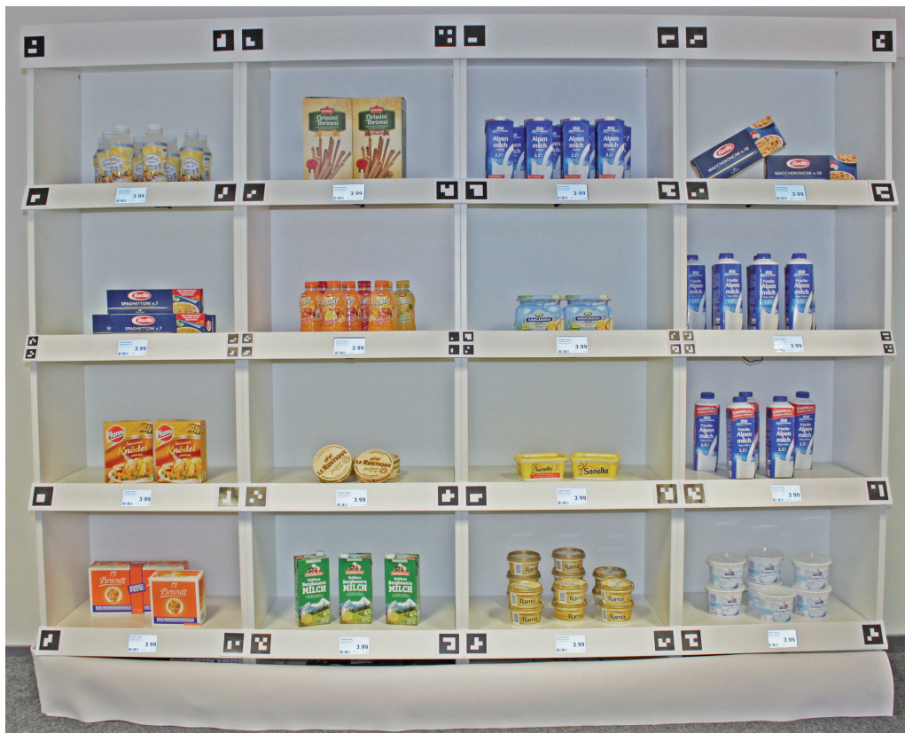
Figure 5.4: Representation of the shelf, which was created to guide the gaze. Smartphones, of which only the displays are visible, serve as price tags/actuators. 2D barcodes are used by the eye tracker to localize the environment.
