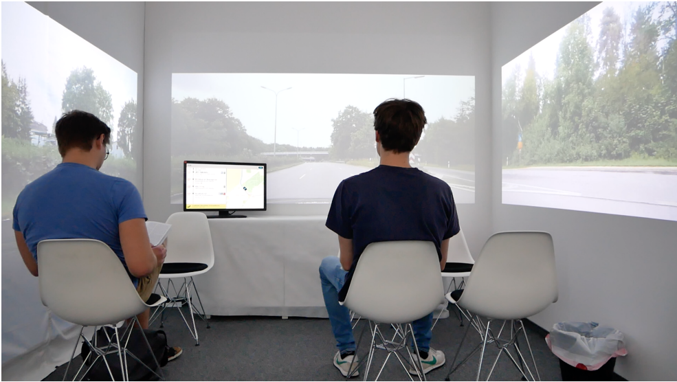
Figure 3.1 – Immersive video-based AV simulator with three video projections and a 26-inch passenger information display. In the conducted user study, an actor (left) joined the simulated ride of the participant (right) to simulate the social context of shared AV rides.
