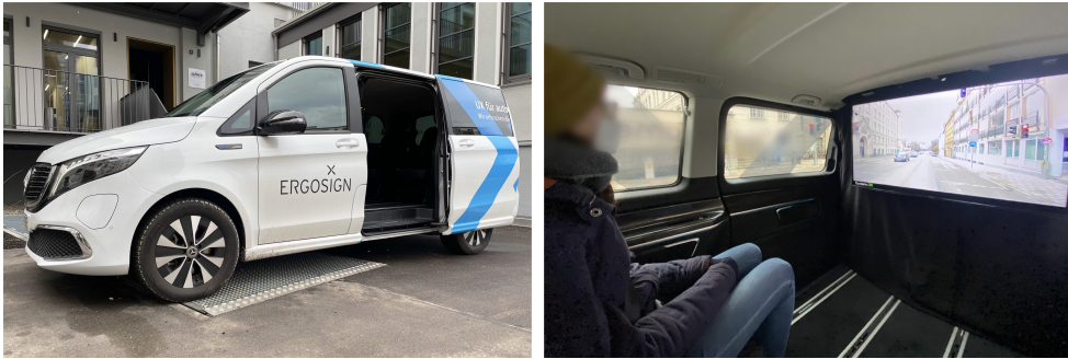
Figure 2.18 – Example of a video-based Wizard-of-Oz setup that we created for our in-vehicle interaction studies (Chapter 4) inspired by the works of Karjanto et al. [131] and Detjen et al. [64].
