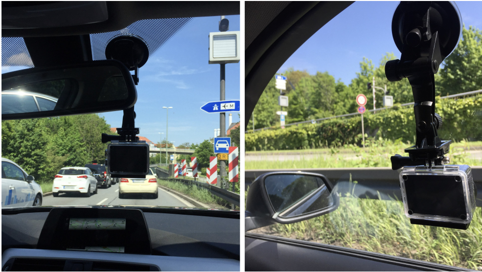
Figure 3.3 – Recording footage of urban traffic for the audiovisual simulation using low-budget action cameras.
