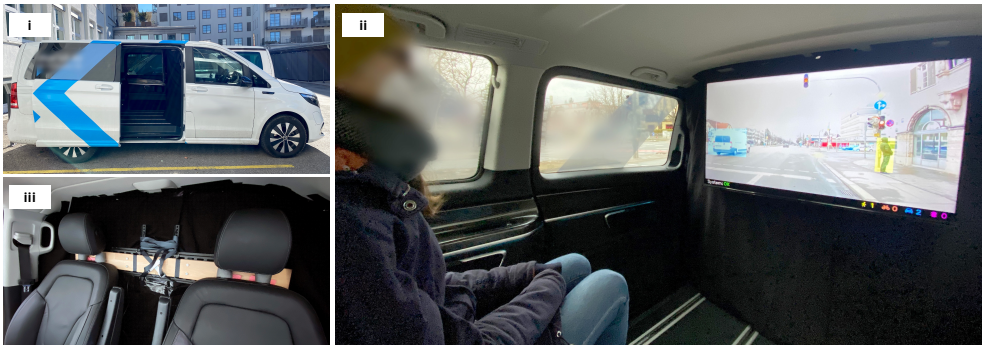
Figure 4.1 – On-road wizard-of-oz prototyping in an electric minivan (i) with a TV mounted on the headrests of the front seats (iii) that displays a video stream from the vehicle’s windshield with AR-based real-time object detection visualization (ii) provided by an embedded computing platform (Nvidia Jetson Nano).
