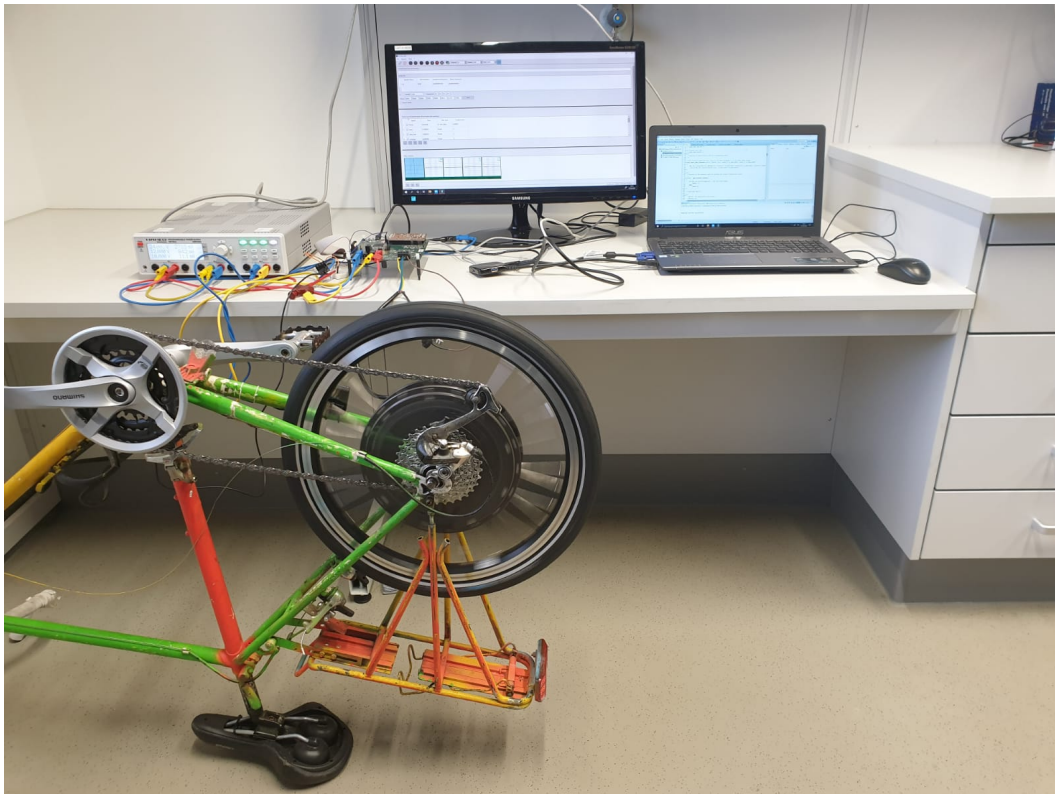
Figure 5.16: Set-up used for the experiments with the e-bike motor.
