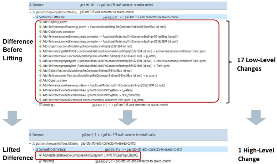
Fig. 1 Semantic lifting can be used to group many fine-grained changes into change sets
