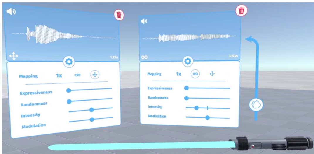
(b) Design of vibrotactile feedback for a virtual lightsaber. Here, a layer with a continuous mapping provides active background vibrations, while a layer using a motion mapping emphasizes the swing of the lightsaber.
