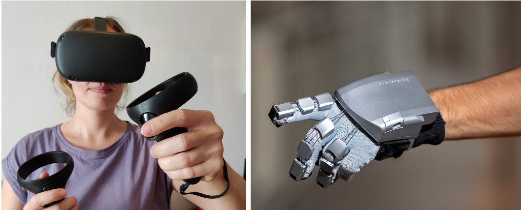
Figure 3.5: VR interfaces with (left) commonly used controllers with basic vibrational feedback, and (right) gloves by SenseGlove able to exert forces onto the user’s fingers (© SenseGlove).
