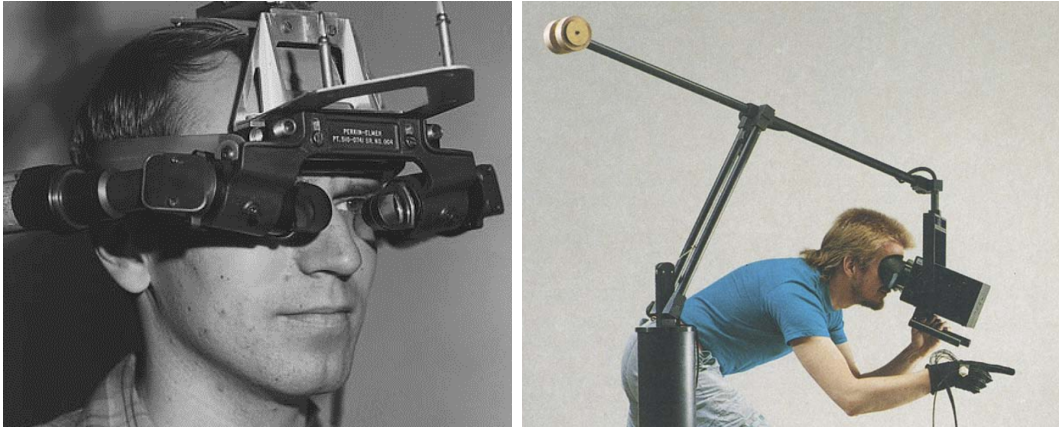
Figure 3.2: A History of Virtual Reality with (left) the “Sword of Damocles” Sutherland (1968), and (right) Binocular Omni-Oriented Monitor (BOOM) from (Bryson, 1992).
