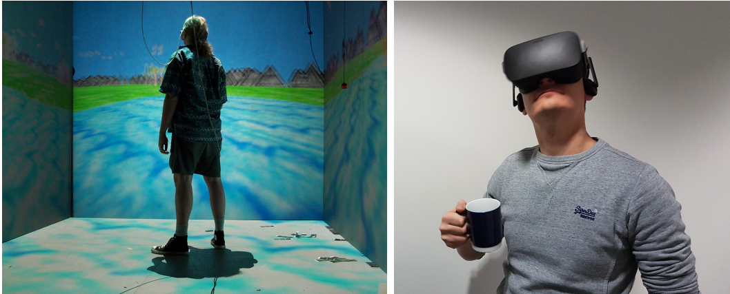
Figure 3.4: VR technologies with (left) a user inside a Cave Automatic Virtual Environment (CAVE) from Wikimedia Commons (2001) and (right) this dissertation’s author enjoying a cup of coffee while wearing a head-mounted display (HMD).
