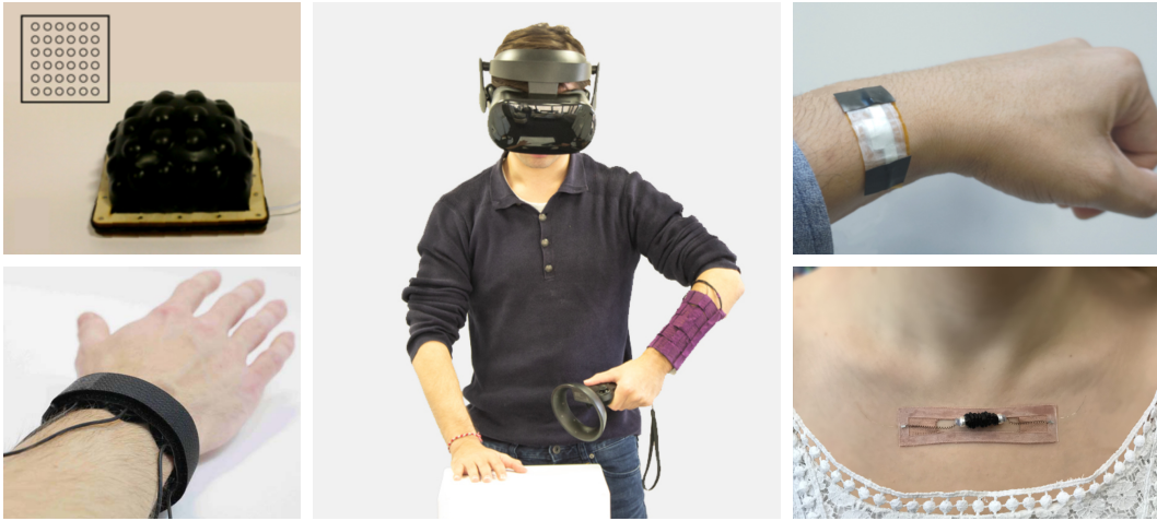
Figure 4.9: Examples of Sensory Integration Approaches, with (left top) a pneumatic interface with surface texture changing properties (Yao et al., 2013), (left bottom) a pneumatic wristband (Young et al., 2019), (middle) an arm-worn SMA-based interface for simulating virtual touch (Muthukumarana et al., 2020), (right top) an on-skin SMA-based soft interface with touch detection in HapSense (Yoon et al., 2019), (right bottom) an on-skin SMA-based interface in Springlets (Hamdan et al., 2019).
