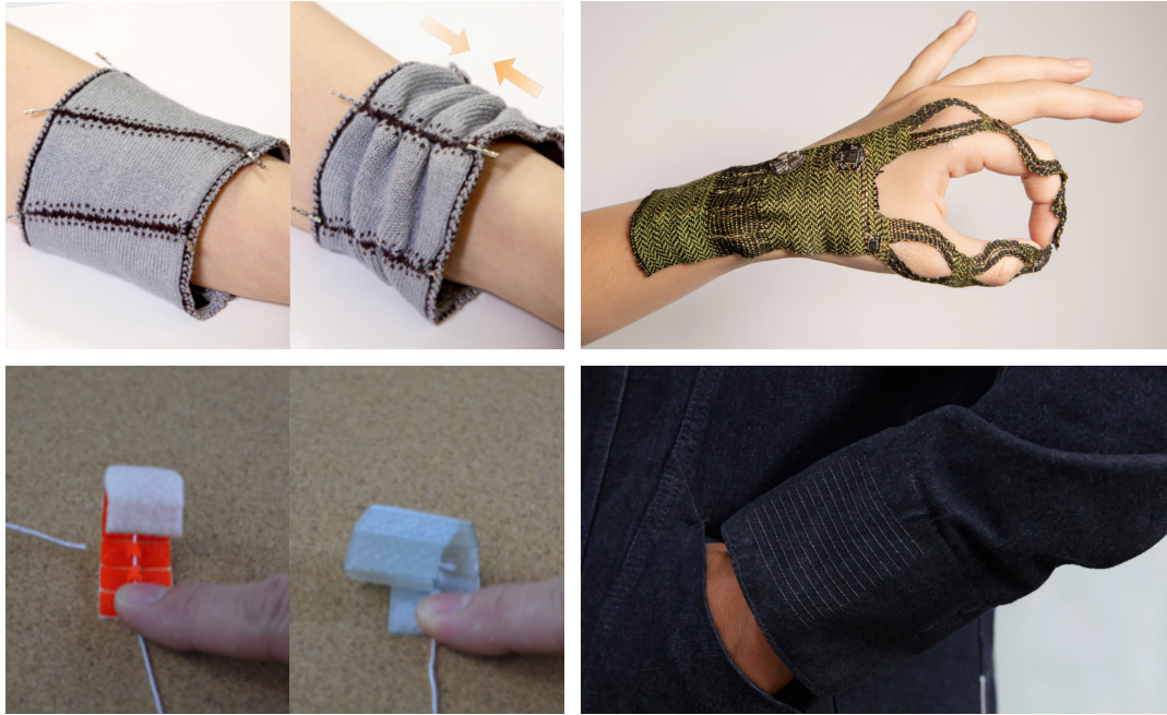
Figure 4.10: Examples of Textile Integrated Haptic Design, with (left top) providing brushing sensations with KnitDermis (Kim et al., 2021b), (left bottom) textile-embedded, string actuated mechanical arms (Rivera et al., 2017), (right top) WovenProbe 's on-skin woven interactive textiles (Huang et al., 2021), and (right bottom) Project Jacquard 's interactive jacket with sensing and vibrotactile feedback (Poupyrev et al., 2016).
