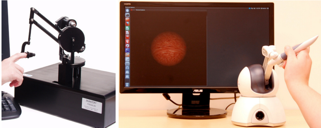
Figure 3.12: Examples of World-Grounded Haptic Interfaces, with (left) the PHANTOM premium configured with a thimble end-effector (© 3D Systems, previously Sensable Technologies), and (right) a SensAble Phantom Omni with a pen-based interface used for exploring virtual textures from Culbertson et al. (2014b).
