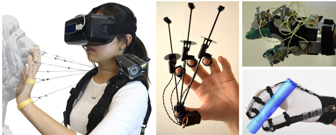
Figure 3.14: Examples of Body-Grounded Haptic Interfaces, with (left) finger and hand strings simulating a virtual statue with Wireality (Fang et al., 2020), (middle) the Wolverine device connecting a user's thumb to other fingers (Choi et al., 2016), (right top) a hand exoskeleton with active motors (Blake and Gurocak, 2009), (right bottom) a more compact hand exoskeleton using electrostatic brakes (Hinchet et al., 2018).
