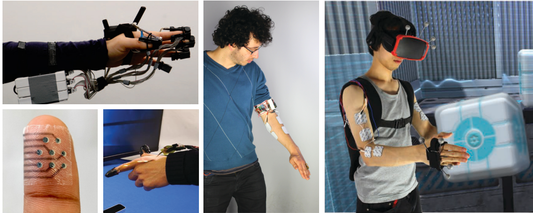
Figure 3.16: Examples of Interfaces using Electrical Stimulation, with (left top) an electro-tactile finger interface (Hummel et al., 2016), (left bottom) on-skin electric actuation in Tact-toe (Withana et al., 2018) next to a combination of mechanical and electrical actuation in FinGAR (Yem et al., 2016), (middle) EMS applied to the user's forearm (Lopes and Baudisch, 2017a), and (right) EMS for simulating heavy objects in VR (Lopes et al., 2017).
