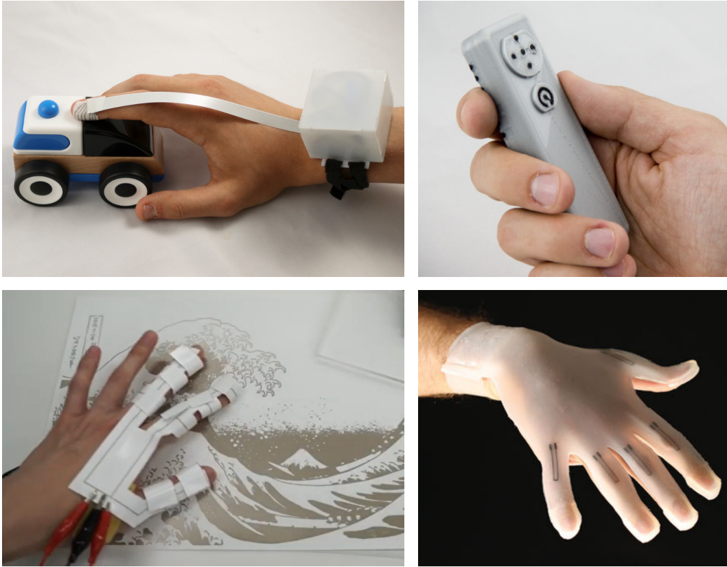
Figure 4.8: Examples of Conductive Haptic Fabrication, with (left top) tactile feel-trough effects (Withana et al., 2018), (left bottom) combined electro-tactile and electrostatic forces (Kato et al., 2018), (right top) tactile pixels embedded inside a 3D printed remote (Groeger et al., 2019), and (right bottom) an on-skin interface (Muth et al., 2014).
