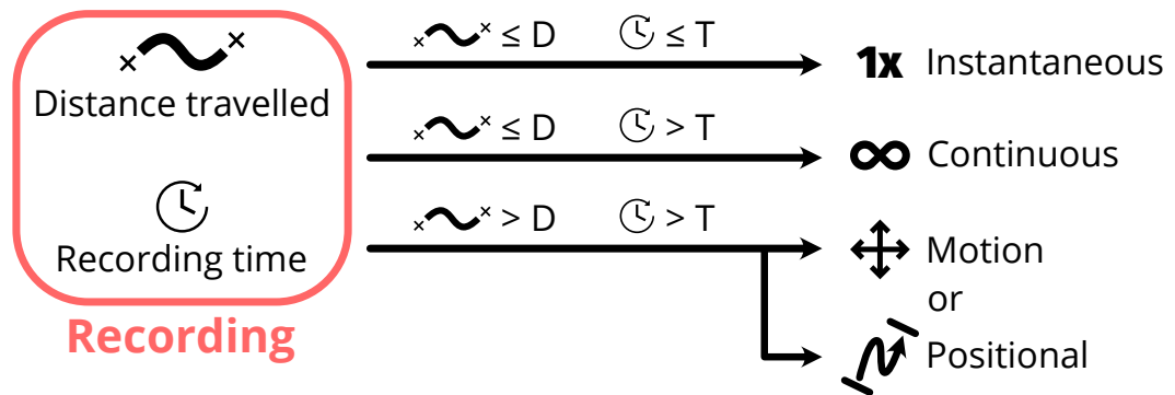
Figure 9.5: The design tool infers the spatio-temporal mapping of a vocalization directly after recording by considering the user's movement magnitude and the recording duration. D (0.5 m) and T (2.5 s) are empirically determined constants.
