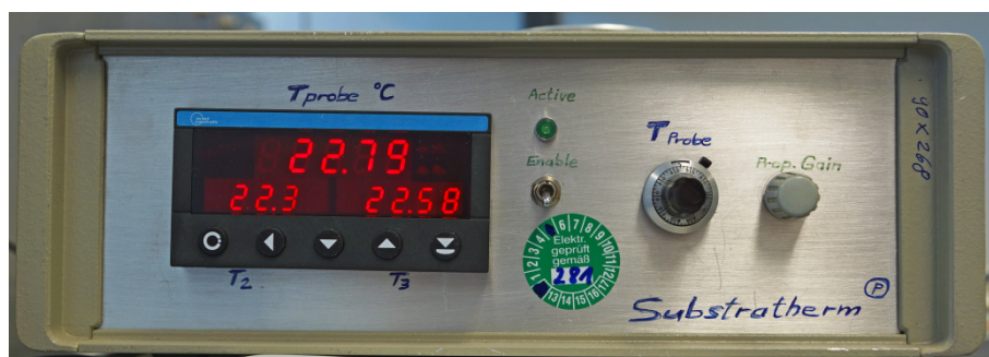
Fig. 11-5 Front view of the SubstratTherm controller for the substrate temperature. T_2 = gas temperature inside the reactor; T_3 = gas temperature at the evaporation stage entrance.
