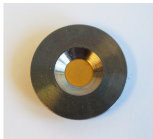
Fig. 3-3 Top view of the quartz crystal holder with attached QCM quartz.
