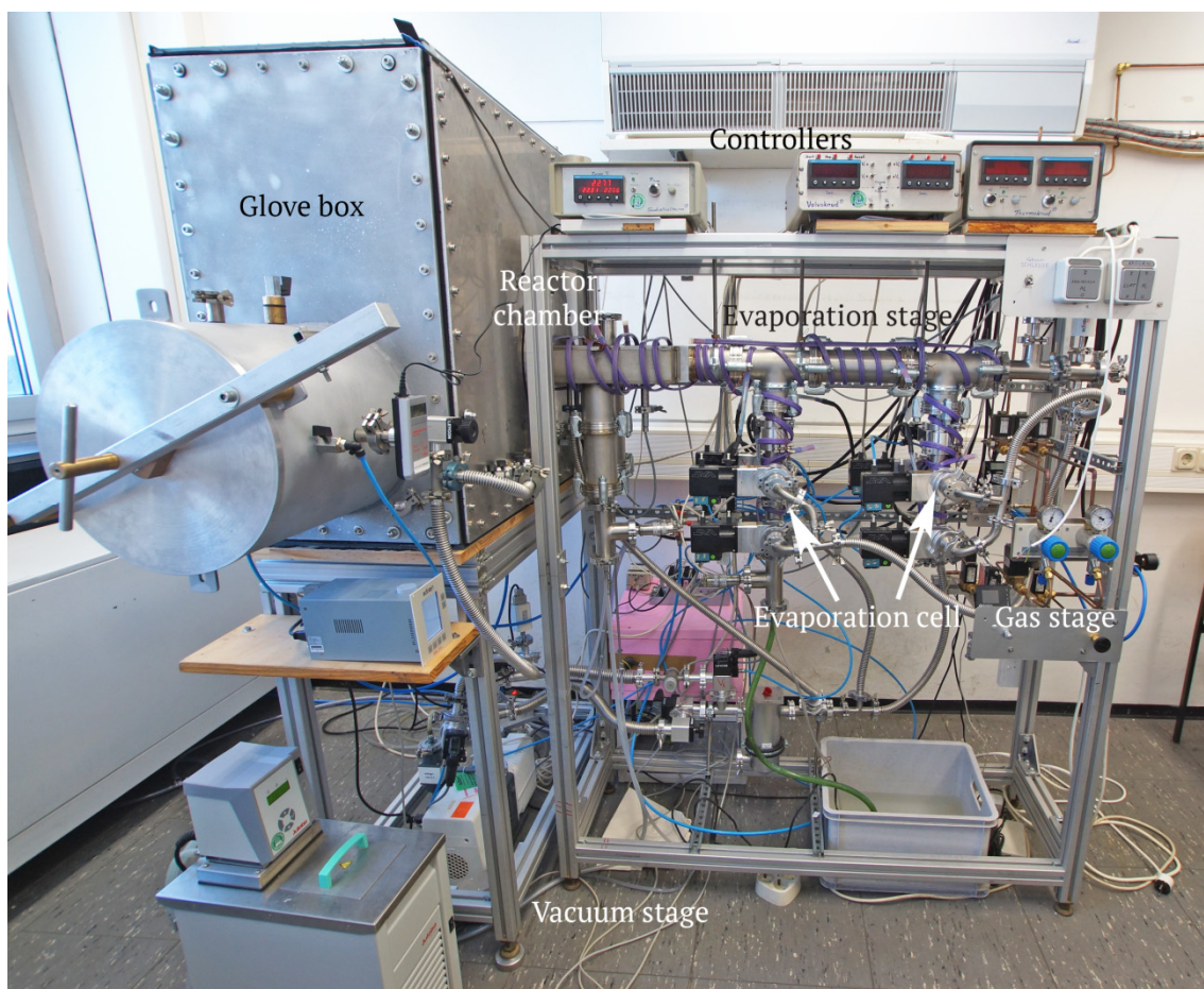
Fig. 4-3 View of the customised MLD apparatus without wall pipe insulation.
