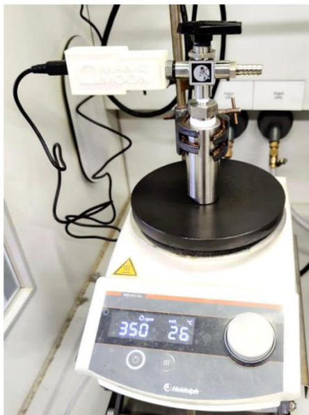
Figure S1. Man on the Moon X103 ® kit in a typical kinetic gas evolution measurement.
