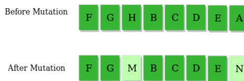
Fig. 2.3 An example of the mutation operator to mutate the gene of an individual.
