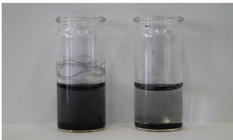
Figure 66 - Catalyst ink 30 min after the end of sonication: left - pristine 10%wtPt/C; right - SCILL (10%wtPt/C+IL2)
