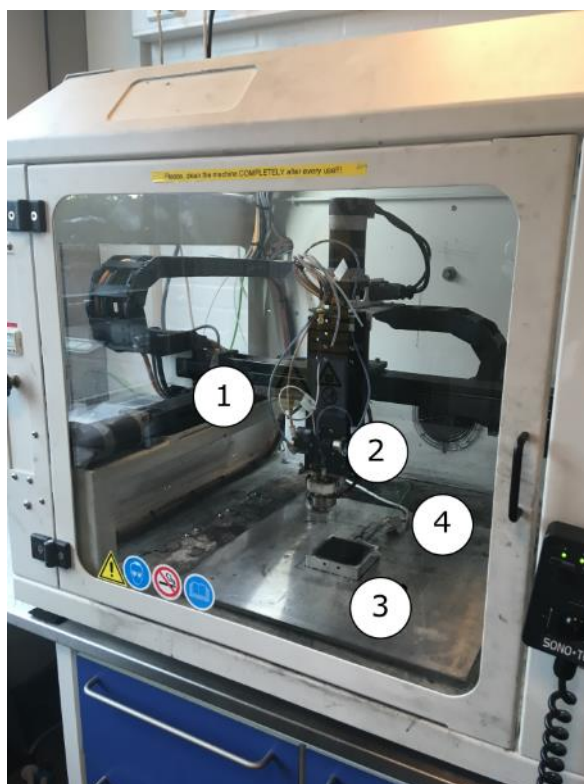
Figure 24 - Spraying robot (property of DTU Energy, Lyngby); (1) robot's moving arm; (2) ultrasonic nozzle; (3) heating plate with a sample fixed on the top and (4) heating rods connected to the plate. Ink is pumped by the glass syringe purchase from Trajan Scientific and Medical
