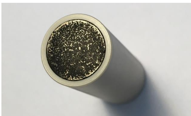
Figure 65 - SCILL deposited on glassy carbon by evaporation of a droplet
