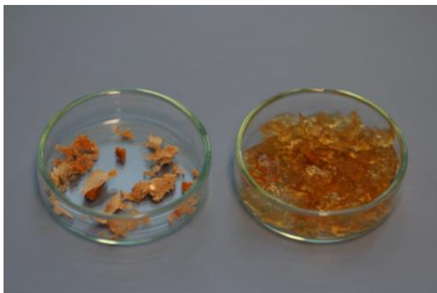
Figure 71 - Modified PBI: left – dry; right – after water uptake
