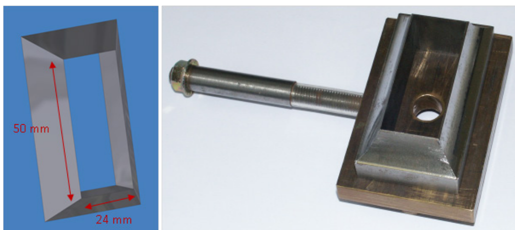
Figure 3-28: Hollow punch for cutting the PTFE spacers [135]
