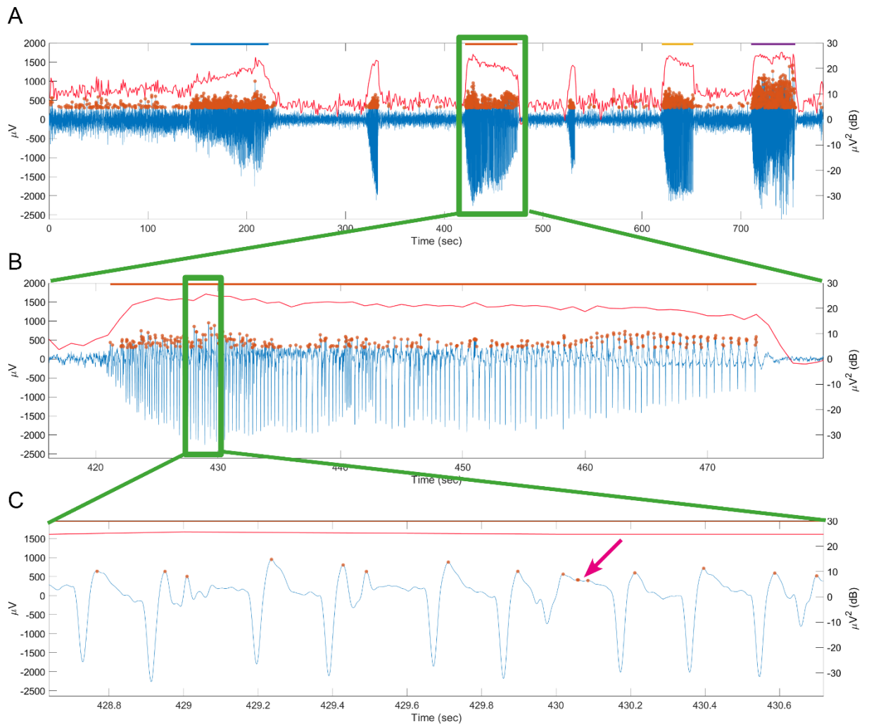
Figure 34: EEG spike-train analysis. A) Four spike trains fulfilling the detection criteria were discovered (colored bars). B, C) Magnification of the second spike train makes it possible to identify individual spikes, and shows that all major amplitude peaks were detected correctly. C) Detailed view of the EEG signal, revealing two false positive spikes (arrow).
