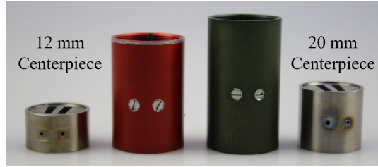
FIGURE 2.7: Double sector AUC cells with different centerpiece thicknesses.
