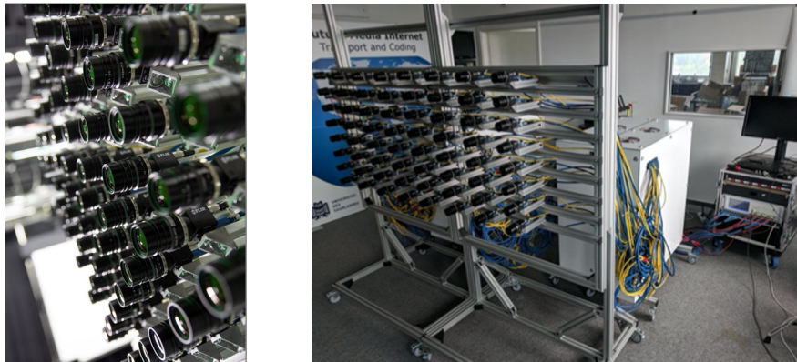
FIGURE 2.11: The 5D light field camera array
