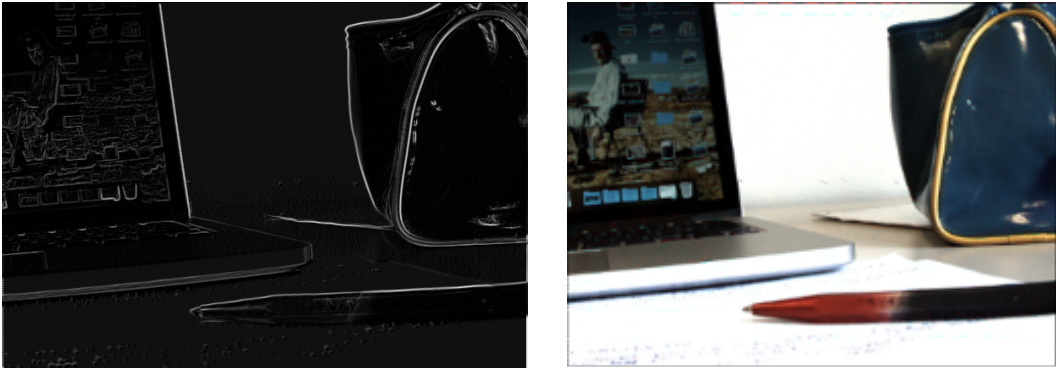
FIGURE 4.12: Center view of the Desktop light field image; a) Reconstructed view after maximum weighted average of luminance; b) JND based Gaussian filtered view
