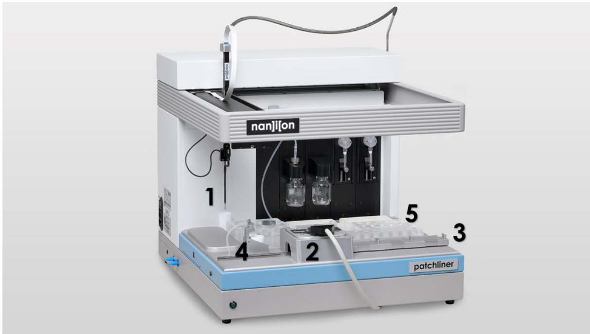
Figure 2.2 Patchliner set-up. Image adapted from Nanion website: https://www.nanion.de/en/products/patchliner.html . The Patchliner consists of: (1) a roboting pipette to aspirate/dispense solutions, cells and compounds; (2) a measurehead, where the patch clamp experiments take place; (3) a chip wagon accommodating up to three chips at a time; (4) a cell hotel, containing the cell suspension; (5) a compound storage area with bottles, glass tubes and Eppendorf.
