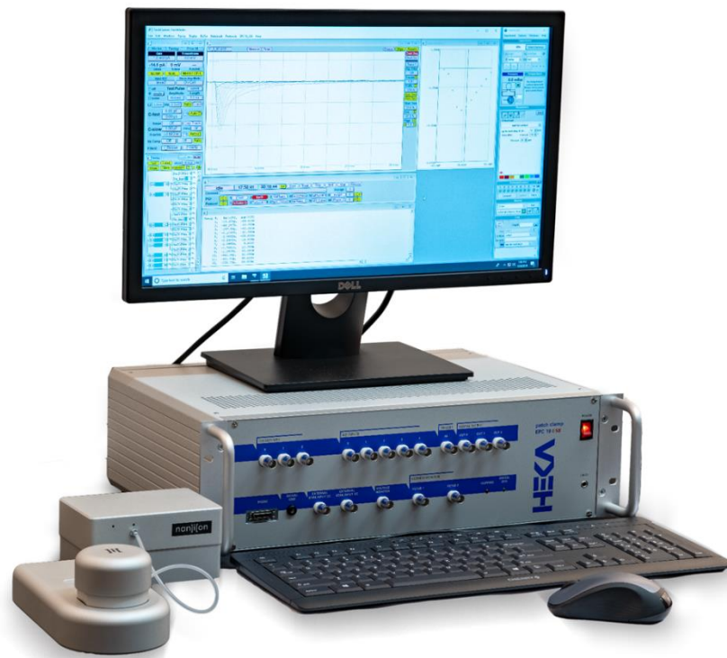
Figure 2.1 Port-a-Patch basic set-up. Image taken from Nanion website: https://www.nanion.de/en/products/port-a-patch.html . A basic planar patch clamp set-up equipped with a Port-a-Patch, an amplifier (HEKA Elektronik) and a computer.
