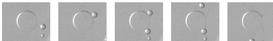
**Figure 1.** Time series of droplets being hydrodynamically attracted to circular PDMS pillars (1 mm in diameter) before phase separation and delivering ethanol during phase separation. After phase separation, the remaining droplet leaves the PDMS target and self-propels away from the circular pillar. The corresponding movie is available in the supplementary information.
