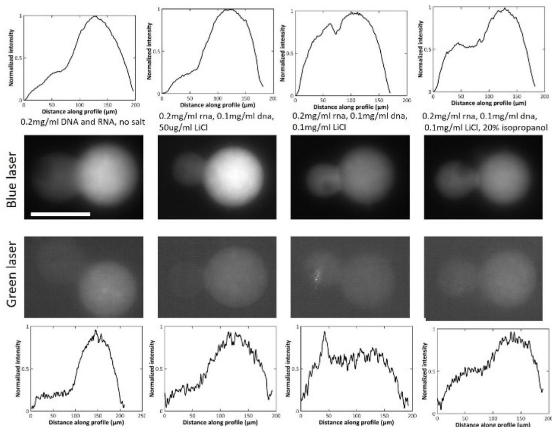
**Figure 5.** Fluorescence pictures of a active Janus active droplet with sDNA and RNA and as a function of different salt composition and concentration. The sDNA and RNA fluorescent sensor is acridine orange (AO, 10  $\mu\text{g/ml}$ ). The upper row shows the fluorescent images under blue laser illumination (473 nm), which detect RNA. The upper row shows the fluorescent pictures under green laser illumination (532 nm), which detect DNA
