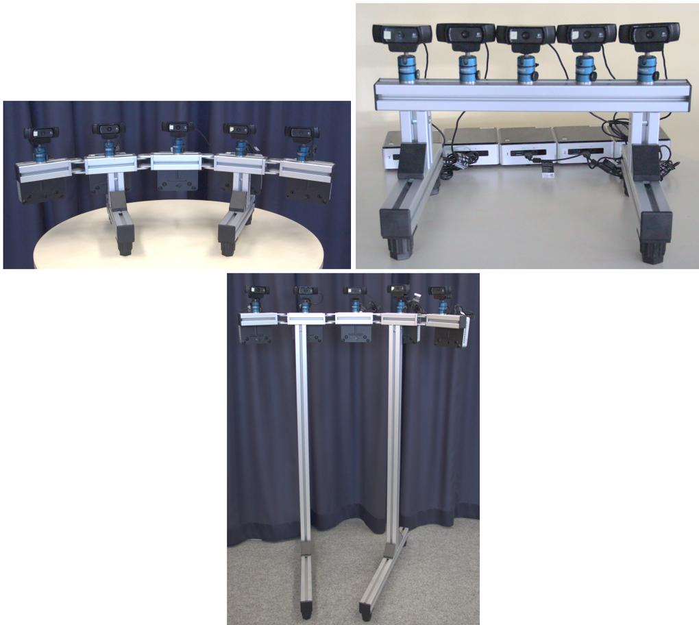
Figure 2.7.: Mounting options for the array with long and short legs and varying options for horizontal placement
