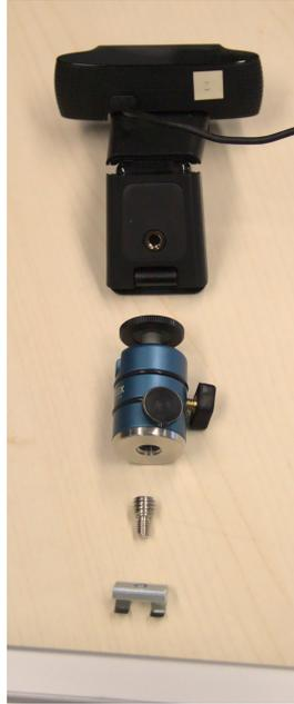
Figure 2.8.: Mounting mechanism for the cameras
