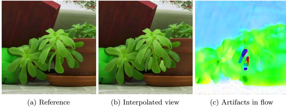
Figure 6.6.: Optical flow results for interpolation artifacts.
