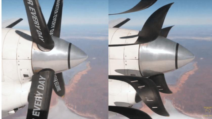
Figure 2.1.: Differences between global (left) and rolling shutter (right) in images of a spinning airplane propeller.
