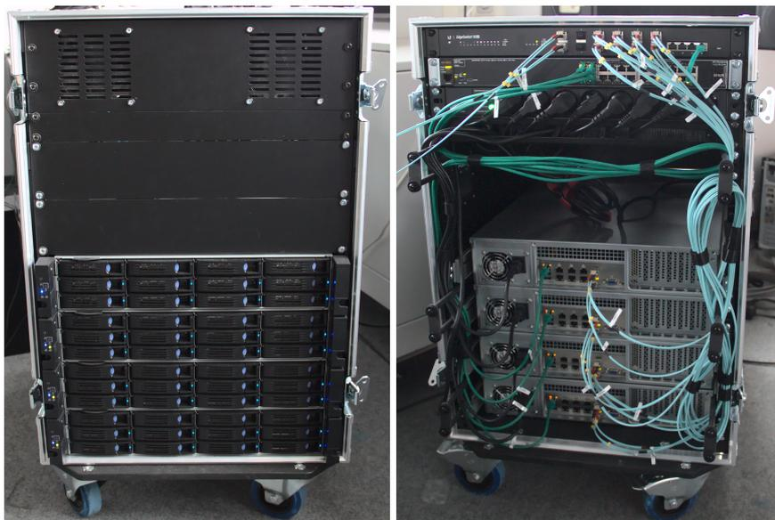
Figure 2.27.: Front and back views of the storage cluster case with all connections
