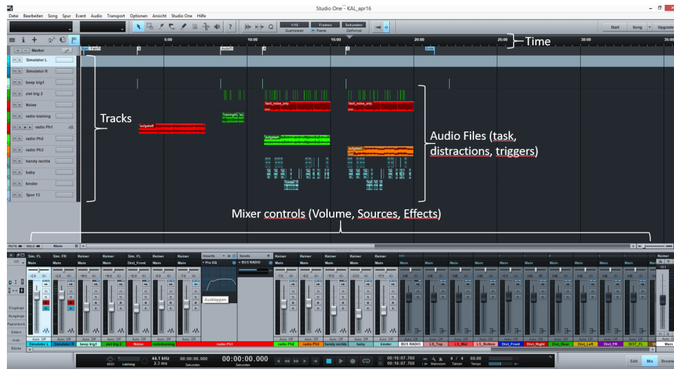
Figure 2.3: Studio 1 software overview. The software allows to split tasks, distractions and triggers into different audio tracks and control both the volume and the directionality of each one separately. Each track can be assigned to one or several of the 24 speakers in the system.
