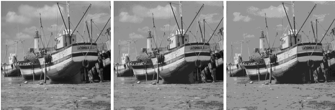
Figure 1.6: Example of swarm-based quantisation. Left: Original image from [Sig15] with 255 greyscales. Centre: Quantised image with 16 greyscales. Right: Quantised image with 8 greyscales.
