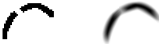
Figure 3.6: Idea of coherence enhancing image filtering. Left: input image showing an interrupted curve. Right: filtered image with closed gap.
