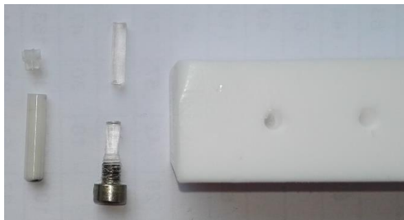
Figure 214: Teflon mould for curing elastic polysiloxanes to receive a rod which can be placed inside the zirconia solid-state NMR rotor.
