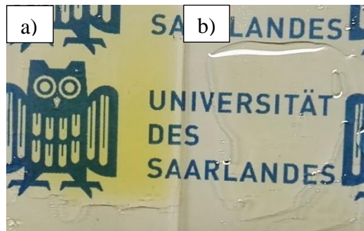
Figure 102: Images of the cured 10.0 wt% ZrO 2 containing MA6.3_MM37.5_PP37.5_TP18.7, a) after curing and b) after exposure to 450 nm light for three days.
