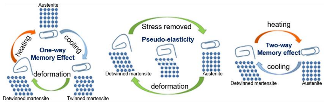
Figure 1.3: The three main effects in SMA materials. (Left hand side) One-way shape memory effect. (Center part) Pseudo-elasticity memory effect. (Right hand side) Two-way Memory effect.
