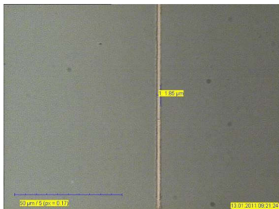
(c) Smallest test patterns obtained after Pt liftoff.
