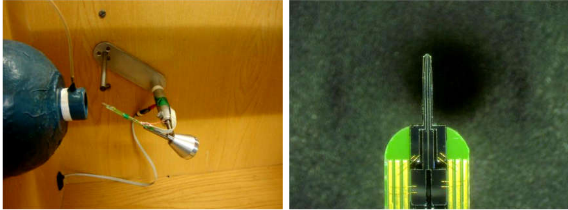
(d) A hot wire attached to a rotary arm at 45° pitch. (e) A hot wire with the sub-mounting package.
