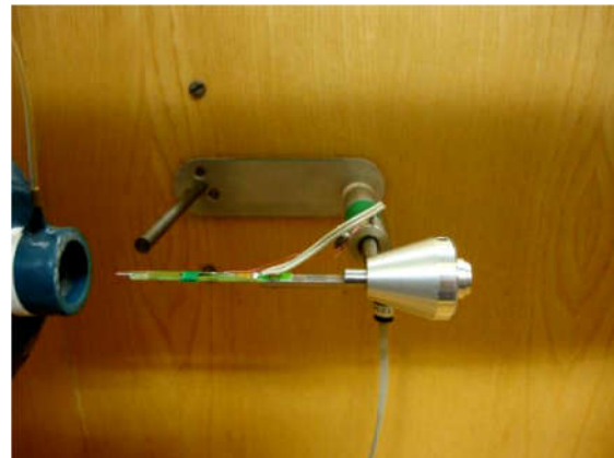
(c) A hot wire attached to a rotary arm at 0° pitch.
