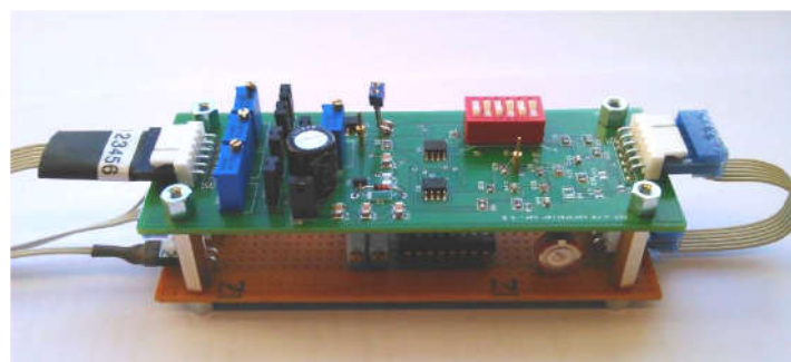
(b) The completed constant temperature circuit.
