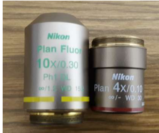
FIGURE 3.3: (a) Image of two different objectives with magnification m = 10 and numerical aperture NA = 0.3 (left) and magnification m = 4 and numerical aperture NA = 0.1 (left).
