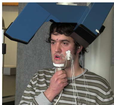
(b) Recording of ultrasound and EMA data. The subject holds the ultrasound probe while sitting in the Carstens AG501 articulo-graph.
