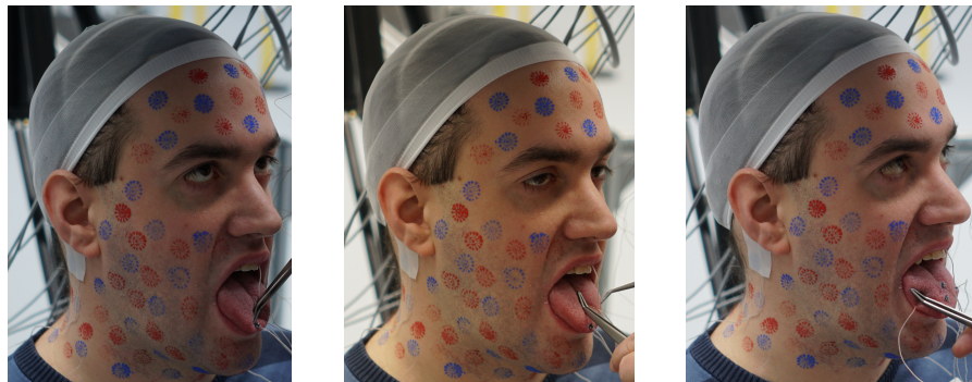
Figure 5.2.: EMA sensor coils are glued to points of interest on the tongue.
