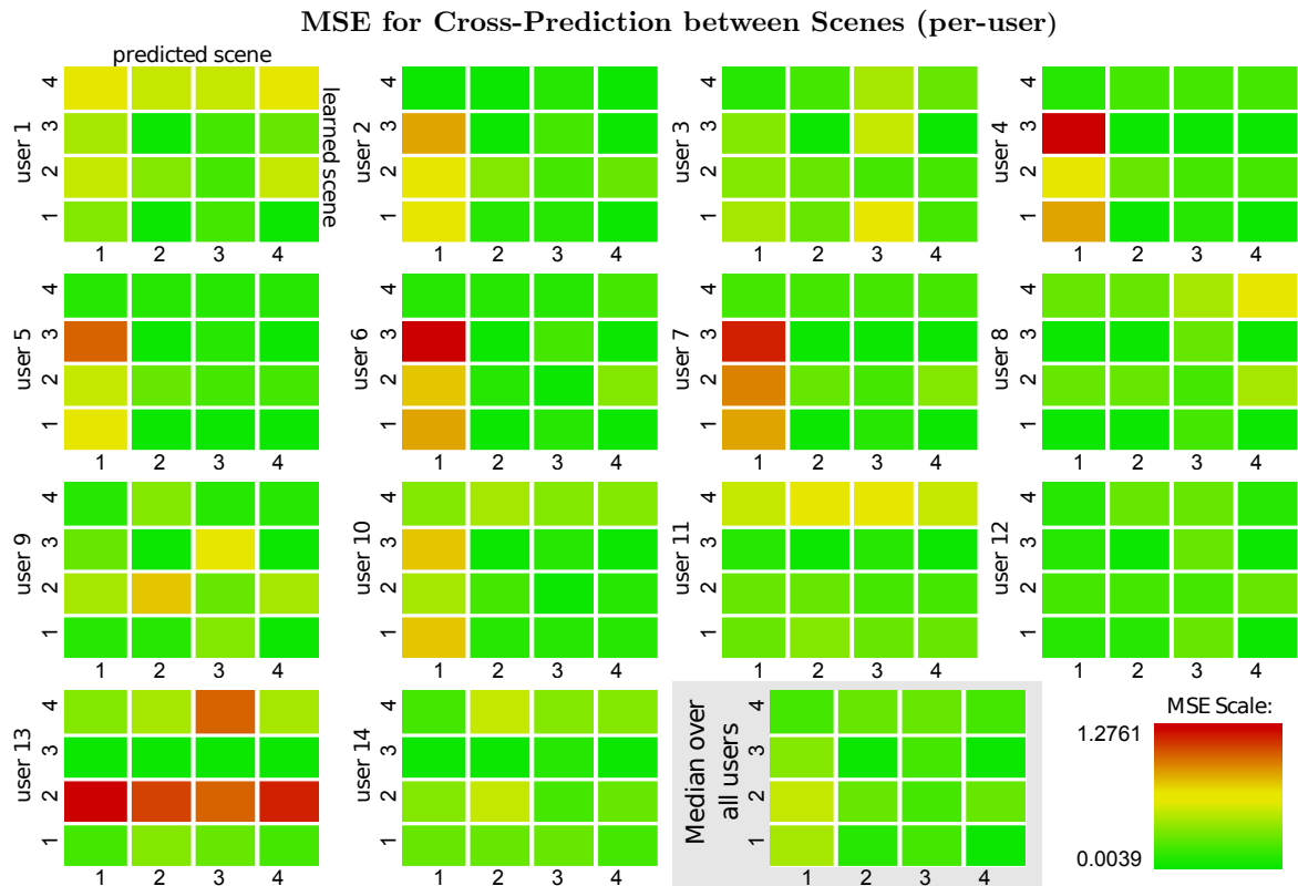
Figure 103: The mean square error (MSE) in meters when training each of the 14 individual users across scenes (1=Sponza, 2=TestNear, 3=TestFar, 4=Study). Rows represent learned scenes, columns represent predicted scenes. A total of 50% of the data per trained scene was used for building the model. The MSE was computed for all training samples of the respective predicted scene.
