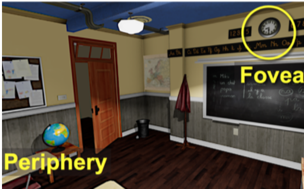
Figure 46: Image from the foveated renderer by Patney et al. [Pat+16b]. This system uses multi-resolution shading with quality degradation as a result in the peripheral visual field in preference to computing efficiency. Image from Patney et al. [Pat+16b]
