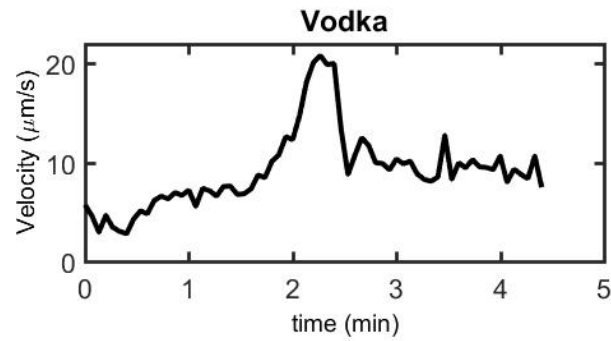
Figure 3.29: Velocity-time diagram of a self-propelled droplet made of Vodka.
