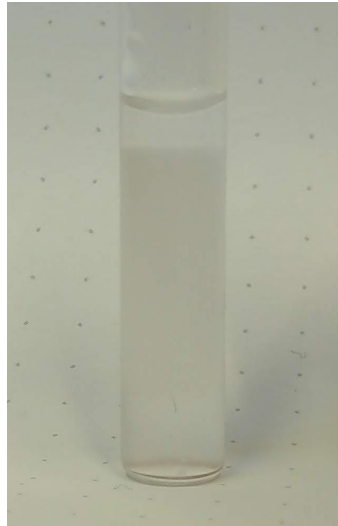
Figure 2.28: Demixing of ethanol and water in bulk. 8 mg monoolein is added to 1 ml 40% ethanol/water mixture (volume percent, for all ethanol/water mixture if not specified).
