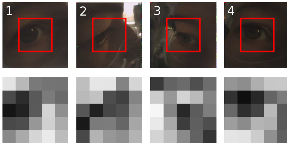
Figure 5.8: (top) Sample eye images from one participant recorded using four NanEye cameras. We identify each of the cameras by the number at the top-left. (bottom) Corresponding cropped low-resolution versions of these images.
