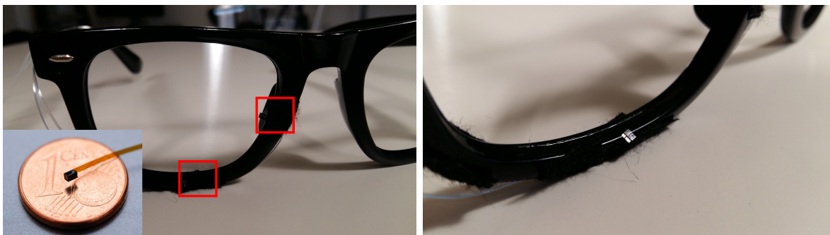
Figure 5.2: Fully integrated version of InvisibleEye consisting of multiple, millimetre-size Awiba NanEye RGB cameras (marked in red) that are invisibly integrated into an off-the-shelf glasses frame. For our evaluations we developed two other prototypes to be able to characterise performance across key design parameters, including image resolution and number of cameras, as well as camera angle and positioning, and to compare with a state-of-the-art (high-resolution) mobile eye tracker.
