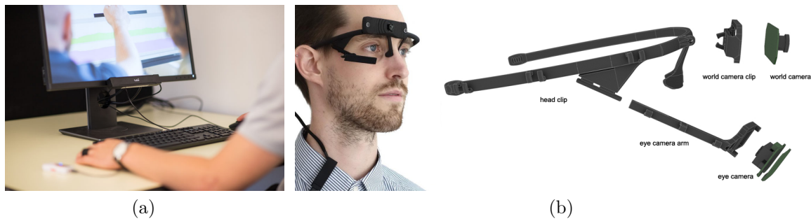
Figure 1.1: Camera-based eye tracking can be differentiated into two methods: (a) remote eye tracking 1 and (b) mobile eye tracking 2,3 .
