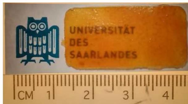
**Fig. 12.** Image of nanocomposite **C6** prepared in a teflon mould.
