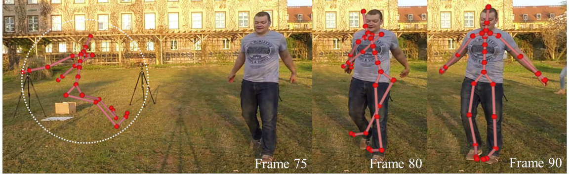
Figure 3.14: Bad pose initialization example. The image shows skeleton tracking resulting from bad pose initialization in the boy_outdoor sequence. Even in presence of strong misalignments, our method is able to successfully recover the correct pose after few frames.
