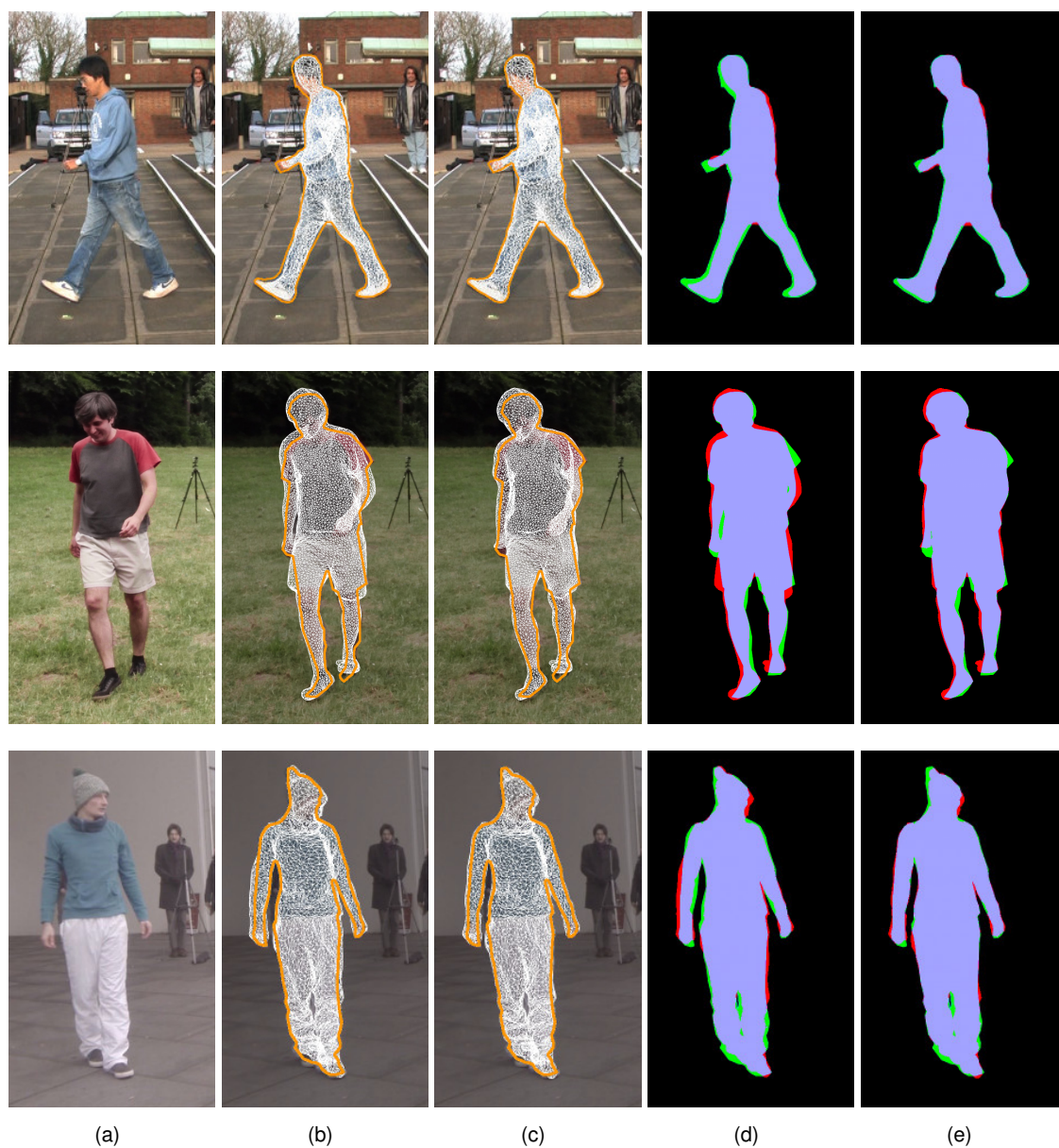
Figure 5.12: Silhouette overlap evaluation in outdoor sequences. (a) Original frame, (b) initial skinned mesh and ground truth contour in orange, (c) final refined mesh and ground truth contour in orange, (d) initial skinned mesh silhouette overlap and (e) final refined silhouette overlap. See Section 5.6.4 for color scheme description.
