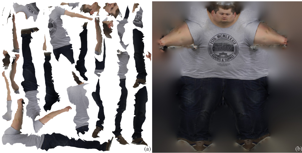
Figure 2.8: Example texture maps. (a) Fragmented texture map and (b) the same texture remapped to a single island.
