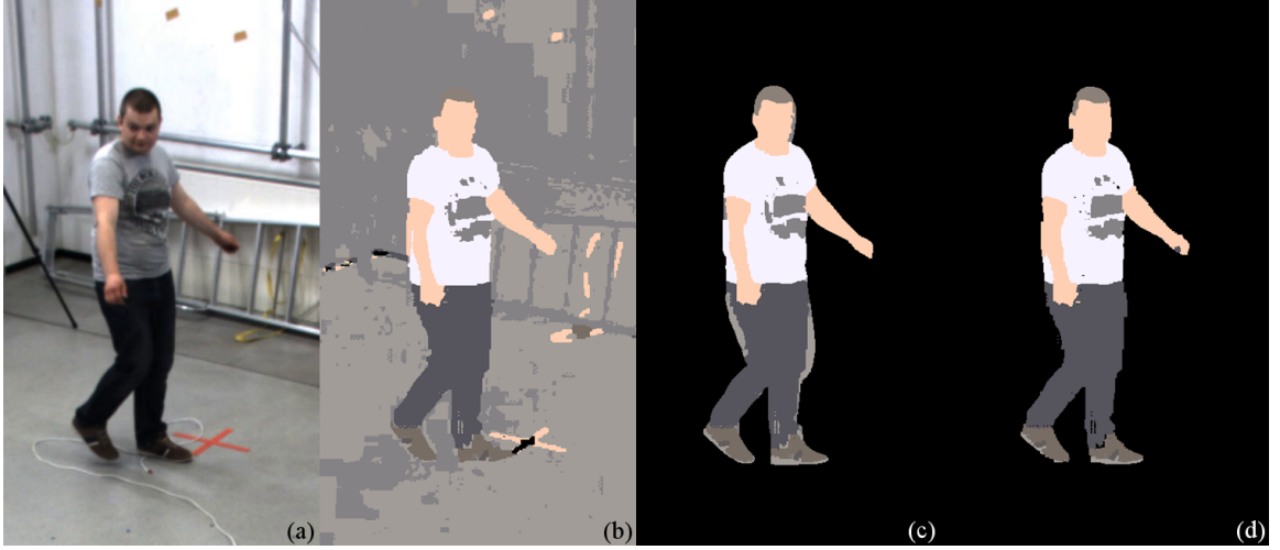
Figure 3.7: Background segmentations using different approaches. (a) Input image, (b) segmentation resulting by assigning background labels the maximum costs (in this case almost no pixel is assigned the background label), (c) segmentation with label costs taken from the pose prior alone (silhouette mismatches arise), (d) segmentation using the proposed background labeling costs.
