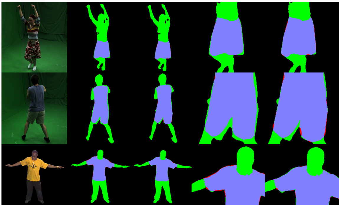
Figure 4.10: Silhouette overlap evaluation of the refined meshes shown for skirt (top), dance (middle) and pop2lock (bottom) sequences. From left to right: input image, silhouette overlap of the baseline (input), silhouette overlap of the refined mesh, zoomed-in baseline overlap, zoomed-in refined overlap. The overlap is estimated from unused views. We used the following color code for the silhouette overlap: Purple: true positives, Green: false negatives, Red: false positives.
