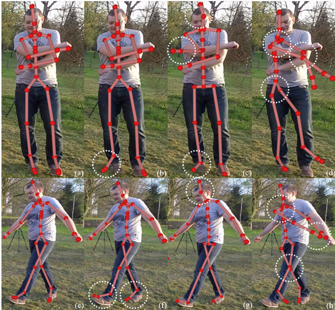
Figure 3.15: Comparison of estimated poses in 2 frames of the boy_outdoor sequence for different methods. (a,e) Our reconstruction, (b,f) Detections-only , (c,g) Image+Detections and (d,h) Images-only . The white circles point to tracking failures.
