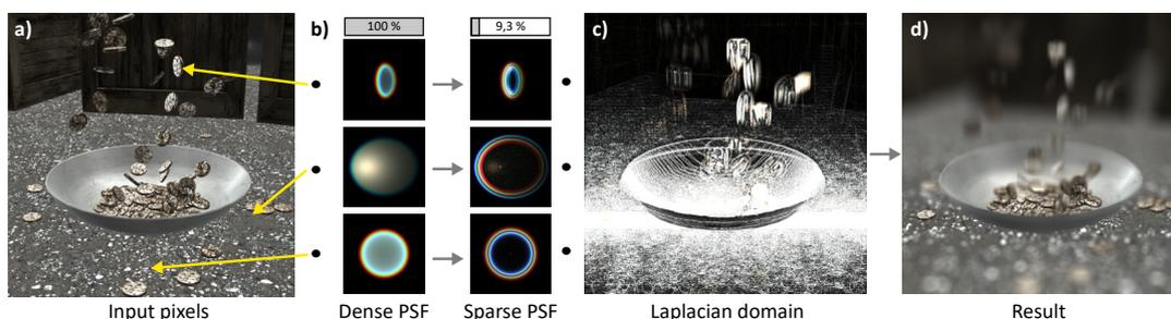
FIGURE 5.1: Computing motion blur and depth-of-field by applying a point spread function (PSF) to every pixel (a) is computationally costly. We suggest splatting a pre-computed sparse approximation of the Laplacian of a PSF (b) to the Laplacian of an image (c) that under integration provides the same result (d). Note the circular bokeh combined with motion blur (1024×1024 pixels, 2 layers, 190 ms, Nvidia GTX 980Ti at .97 SSIM to a path-traced reference).
