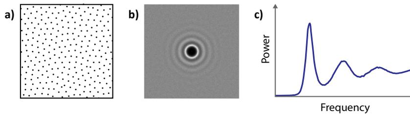
FIGURE 2.7: A sampling pattern (a) is characterized by its expected power spectrum (b) that can be radially averaged to obtain a one-dimensional profile (c). This example shows a blue noise sample pattern, as can be seen from the vanishing energy in the low-frequency region.
