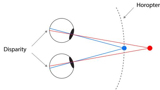
FIGURE 2.3: The geometry of stereopsis. The eyes are converging to the blue point. This gives rise to binocular disparity for the red point, which lies outside the horopter surface.
