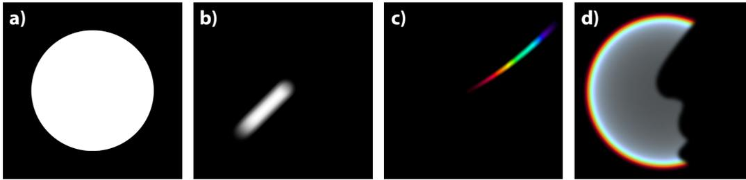
FIGURE 2.5: *Different types of point-spread functions. (a) A circular shape arising from the depth-of-field of a thin-lens camera. (b) A response exhibiting linear motion-blur and depth of field. (c) A spectral response arising from a chromatic aberration. (d) A partially occluded depth-of-field response of a physical lens model.*
