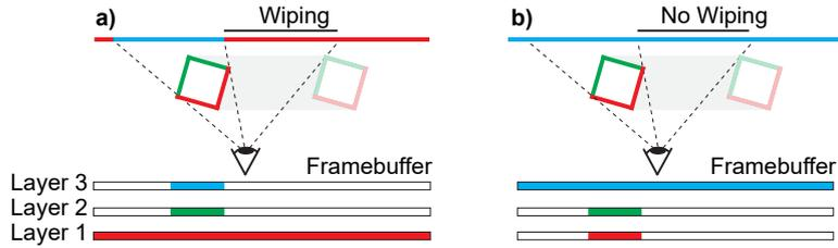
FIGURE 4.9: Per-pixel sorting of layers prevents wiping, here illustrated for a box moving in front of a planar background.
