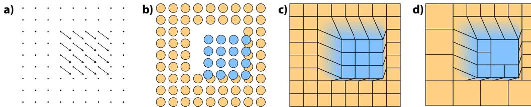
FIGURE 2.6: *Image warping.* (a) *Deformation flow field, resulting in occlusions and disocclusions.* (b) *Point warping.* (c) *Grid warping.* (d) *Quad-tree warping.*
