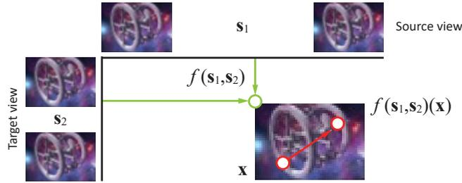
FIGURE 4.4: Common forward flow (red) is a mapping from each image location  $\mathbf{x}$  to a new location  $f(\mathbf{x})$ . We operate on a family of flows  $f(\mathbf{s}_1, \mathbf{s}_2)(\mathbf{x})$  that depend on the source sample  $\mathbf{s}_1$  and the target sample  $\mathbf{s}_2$  (green). In this illustration, the sample space, which is high-dimensional, is depicted two-dimensionally for simplicity.
