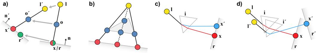
FIGURE 4.5: The geometry of shadow (a,b) and caustic (c,d) flow. (a) A moving light source  $l$ , occluder  $o$ , and receiver  $r$  lead to a moving shadow position  $x$ . (b) Only shadow silhouettes have a unique occluder. (c) A change of wavelength leads to caustic motion. (d) This can be combined with a moving light source  $l$ , dispersive interface  $i$ , and receiver  $r$ . Dashed symbols denote the new configuration.
