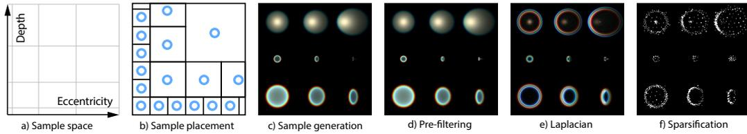
FIGURE 5.4: The steps of our PSF sampling: a) Definition of the sample space. b) Non-uniform placement of samples (blue circles). c) Generation of the PSF at each sample. d) Pre-filtering in the sample space. e) Computing the Laplacian and f) sparsification into a set of points.
