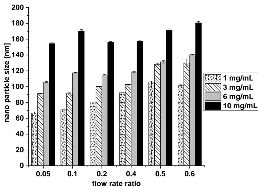
**Fig. 2:** Effect of PLGA concentration on NPs size.
