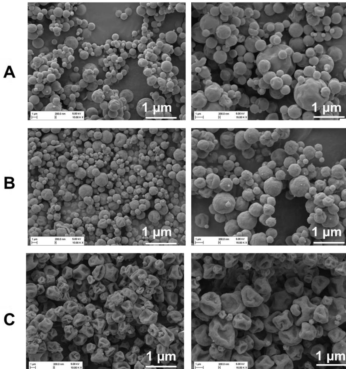
**Fig. 6:** SEM micrographs of spray-dried antibiotics/NAC microparticles. Azithromycin/NAC (A) and Ciprofloxacin/NAC (B), Tobramycin/NAC at, 10.000x and 15.000x magnification respectively.
