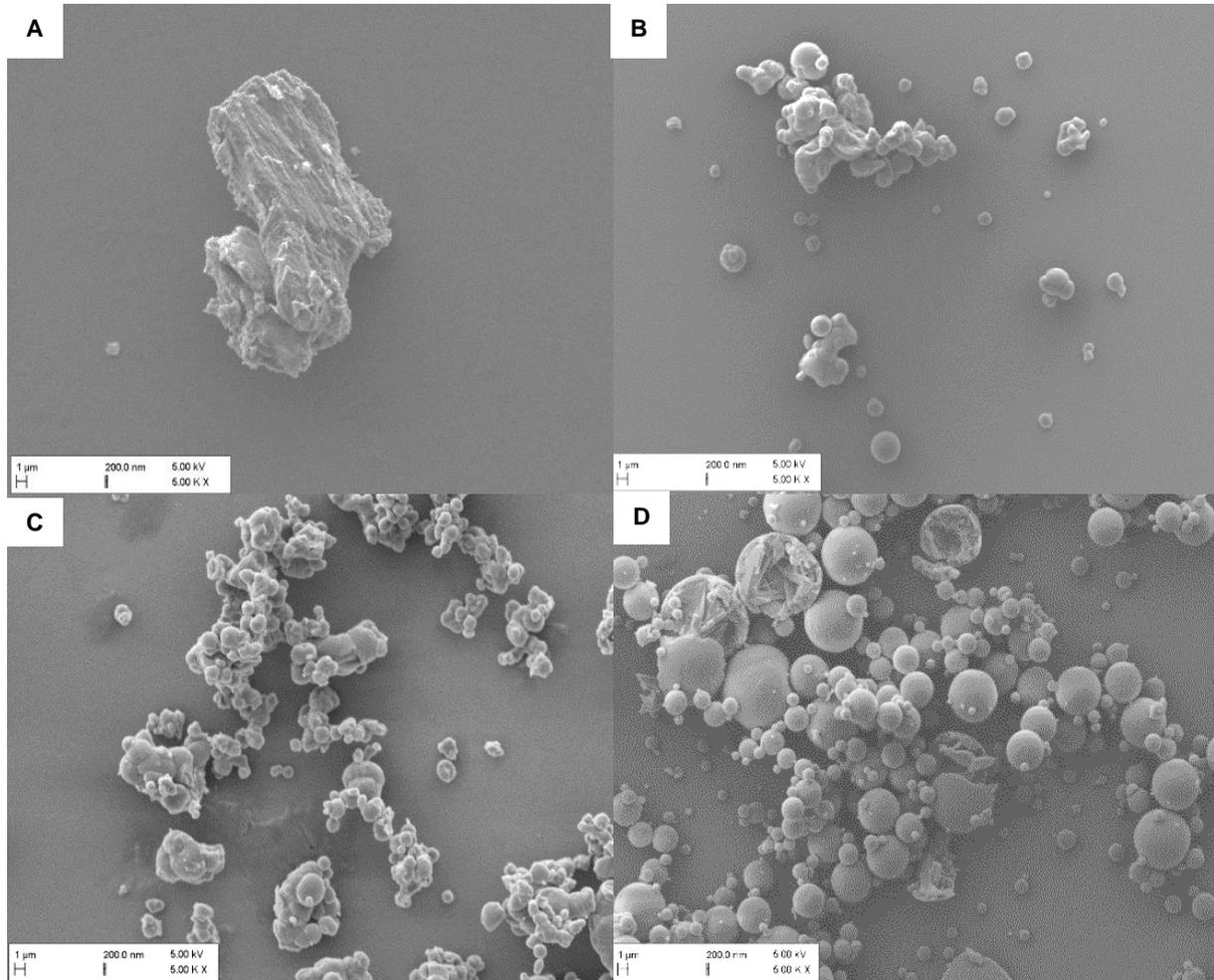
**Fig. 3:** SEM micrographs of spray-dried Mannitol/NAC microparticles. 1:1 ratio (A), 12:1(B), 25:1 (C) and pure Mannitol as reference (D) at magnification 5.000x.
