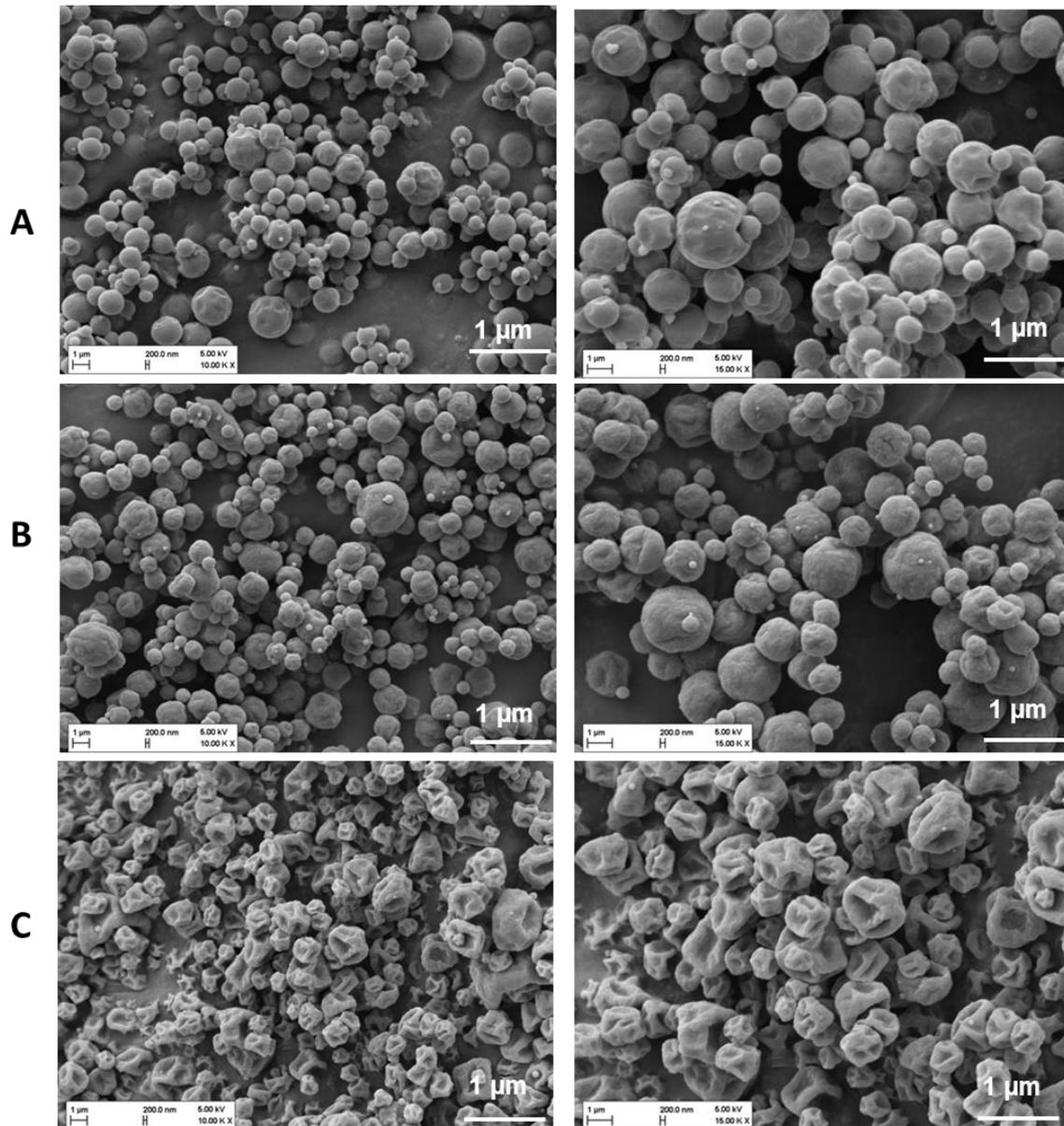
**Fig. 1:** SEM micrographs of spray-dried antibiotics /NAC microparticles. Azithromycin/NAC (A) and Ciprofloxacin/NAC (B), Tobramycin/NAC at, 10.000x and 15.000x magnification respectively.
