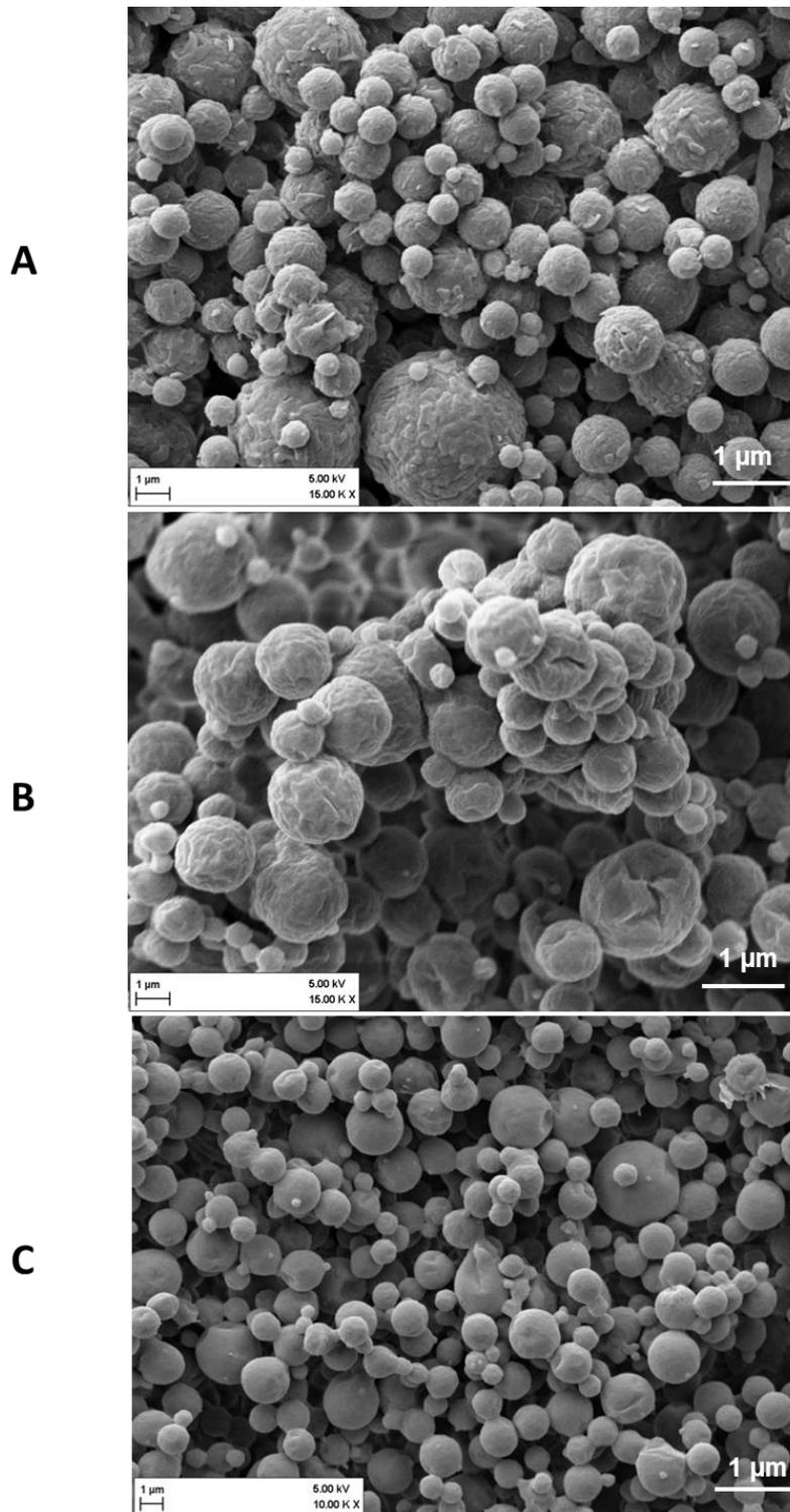
**Fig. 9:** SEM micrographs of spray-dried of (A) Cipro/NAC, (B) Azith/NAC, (C) Tobra/NAC after 3 weeks at 15.000 magnification.
