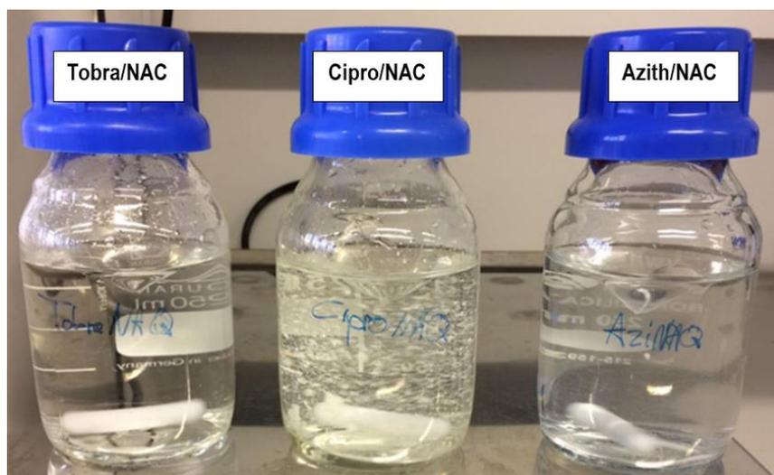
**Fig. 4:** The dry substances of Tobra/NAC, Cipro/NAC & Azi/NAC respectively, show differences in dissolving speed upon contact with water. Cipro/NAC takes longer to completely dissolve than the other two formulations. Finally, all formulations were clear solutions. Picture was taken 1min after contact.
