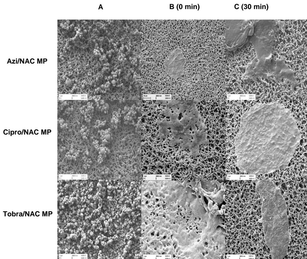
**Fig. 7:** SEM micrographs of spray-dried microparticles deposited on top of a nitrocellulose membrane (A) formulation without placing on top of agarose Pads. (B) antibiotics/NAC at 0 min when got placed on top of Agarose pads, antibiotics /NAC at 30 min (C) at 5.000 x, 10.000 and 15.000x magnification respectively
