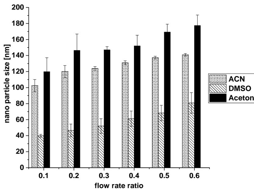
Fig. 5: Effect of solvent nature on NPs size.
