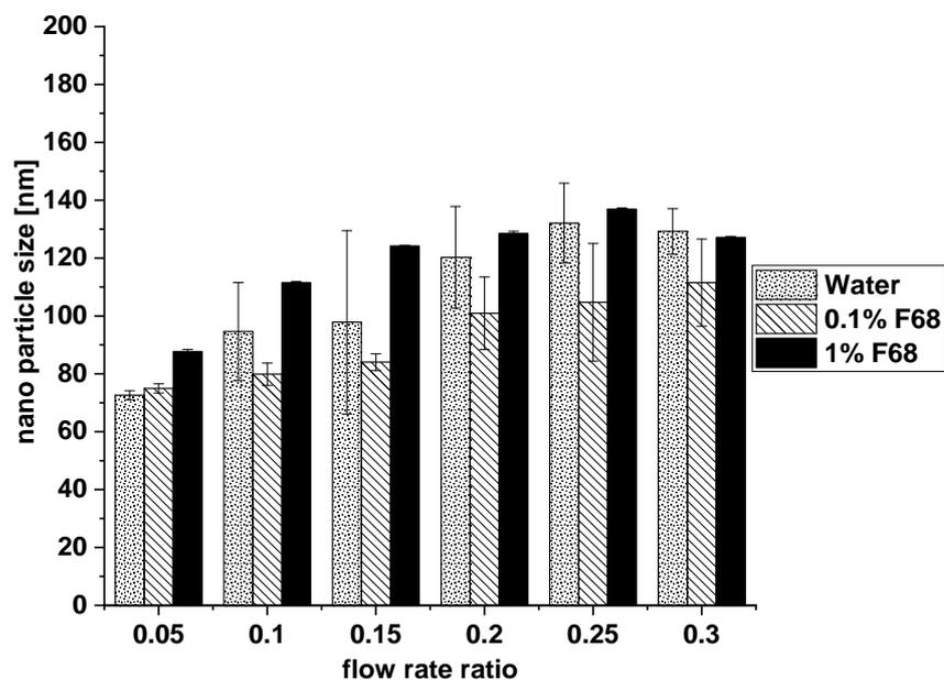
Fig. 4: Effect of stabilizer concentration on NPs size.
