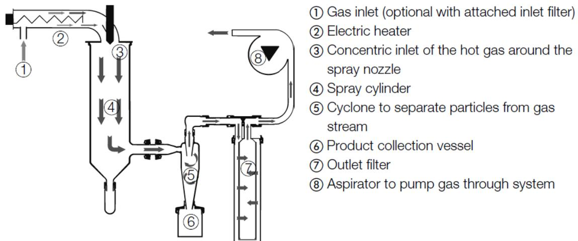
**Fig. 7:** Diagram of a spray dryer, Source: BÜCHI B-290 Manual.
