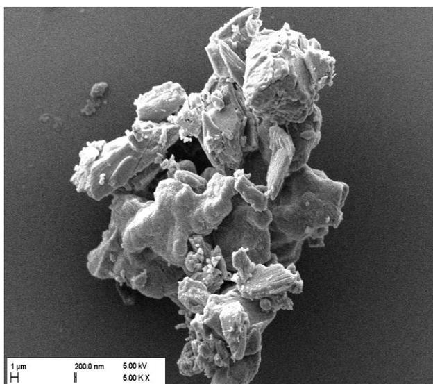
**Fig. 2:** SEM micrograph of pure spray-dried NAC, Magnification 5.000x.
