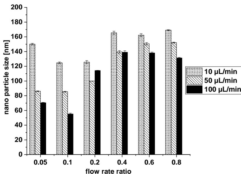
**Fig. 1:** Effect of flow rate ratio and total volume of the aqueous phase on NPs size.
