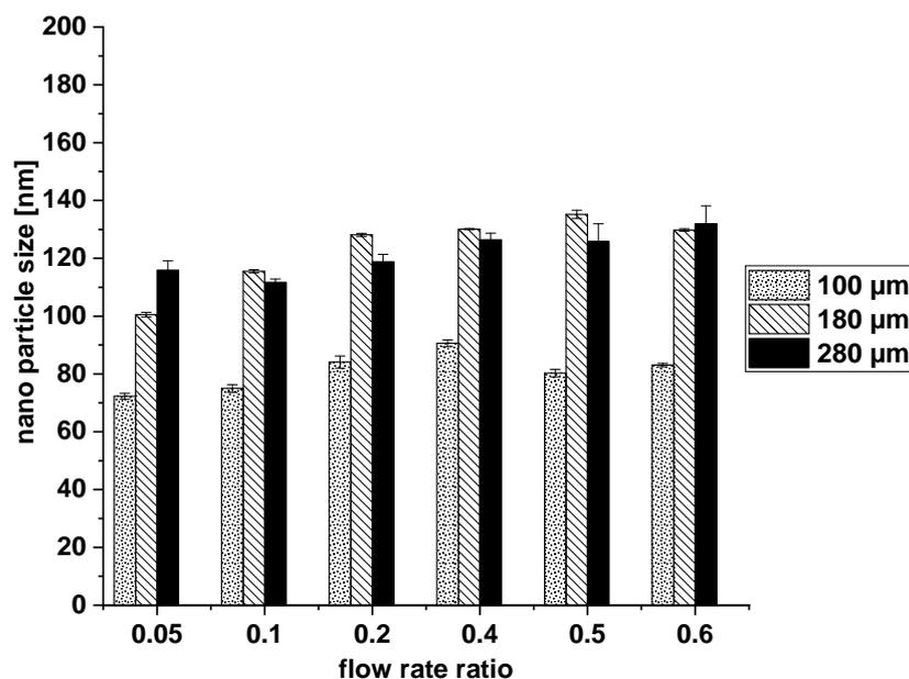
*Fig. 3: Effect of diameter of focusing channel on NPs size.*
