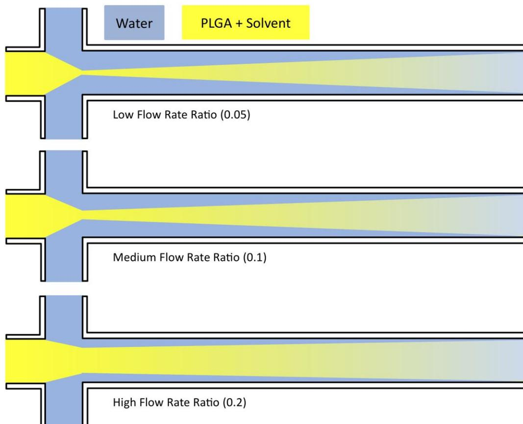
**Sketch 2:** Illustration the impact of increasing the flow ratio on the mixing pattern.
