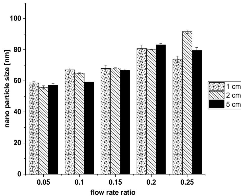
*Fig. 6: Effect of length of the focusing mixing channel on NPs size.*
