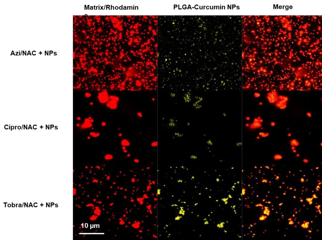
**Fig. 2:** Morphology of co-spray-dried microparticles visualized by CLSM; left row shows the Matrix/Rhodamine B fluorescence, the second represent the fluorescence of the curcumin (nanoparticles) and in the right row the merge of both shown. Scale bar represents 10  $\mu\text{m}$ .
