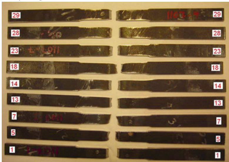
Figure 4-10 Examples of laser welded +Q&P treated tensile test samples.
