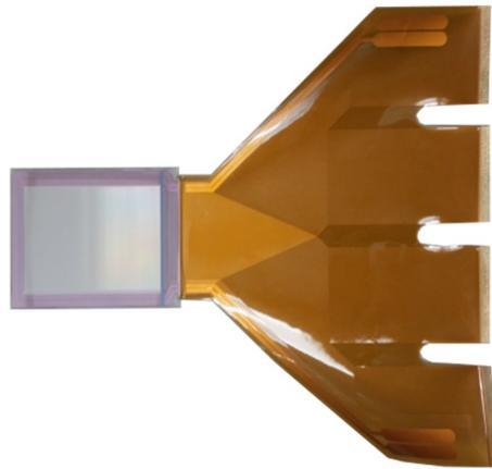
Figure 7-9 2.8" QVGA AMOLED panel from Visionox.
