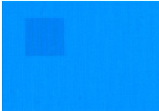
Figure 7-12 Image sticking on AMOLED display (blue OLEDs).
