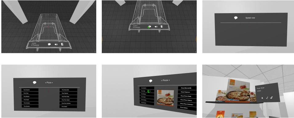
Figure 5.10: **Speech input.** Here, the user starts by gazing at the speech button, and speaks the search term into the microphone. After the search results are displayed, the user can select the desired product in order to be moved to the desired shelf.
