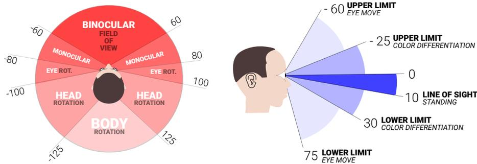
Figure 2.6: Left: horizontal field of view. Right: vertical field of view.
