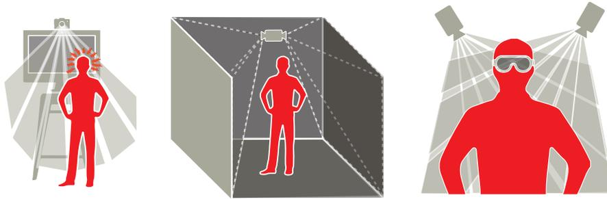
Figure 2.4: Common formats for virtual reality displays. From left to right: fish tank VR, CAVE, HMD.
