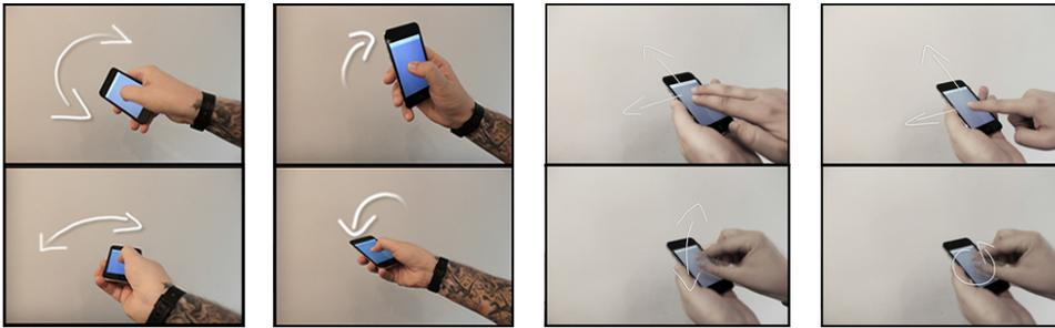
Figure 2.11: Our 3D navigation techniques using smartphone sensors [61], from left to right: tilt, two-finger pan and pinch, and one-finger pan and two-finger rotate.
