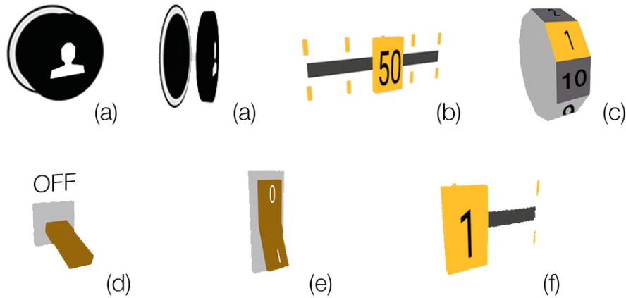
Figure 4.11: Pseudo-haptic UI Menu Control Elements (a: button, b: slider, c: wheel, d: toggle, e: rocker, f: slider switch).
