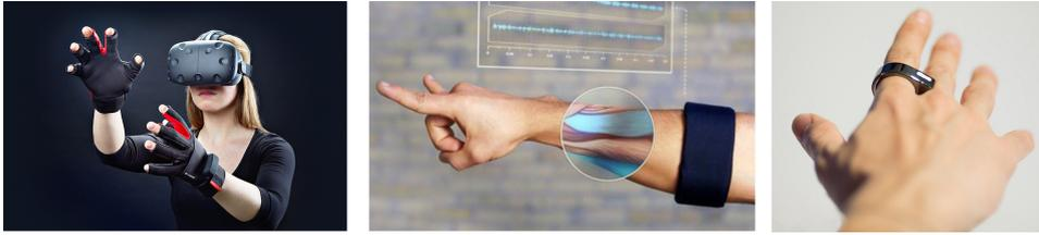
Figure 2.10: Hand-worn controllers, from left to right: Manus VR Glove<sup>25</sup>, Myo Band<sup>26</sup>, and Scroll Ring<sup>27</sup>.
