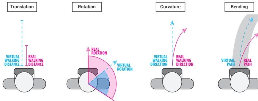
Figure 2.23: Viewpoint manipulation techniques used for redirected walking, adapted from [222]. From left to right: translation [123, 329], rotation [39, 131, 245], curvature [219, 293, 98], and bending [154, 155].
