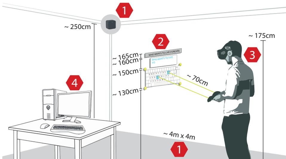
Figure 4.4: This figure illustrates the experimental setup. (1) Vive optical tracker (at  $2.5m$ ) and tracking space with  $4 \times 4m^2$ . (2) Virtual keyboard, stimulus and text input field. (3) Participant wearing Vive and tracked hand-held controllers. (4) PC for experiment control.
