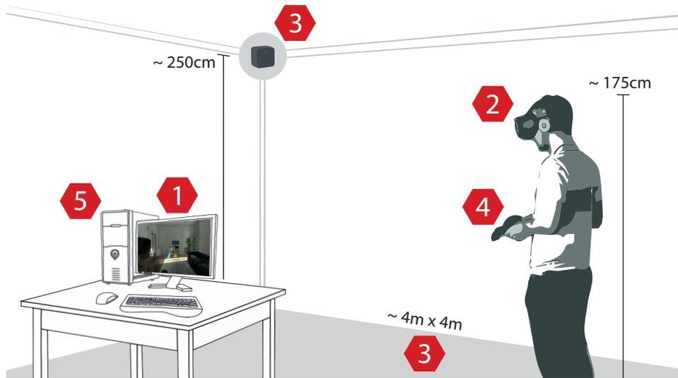
Figure 2.3: Basic components of a VR system. (1) Virtual environment. (2) Virtual reality display, here HTC Vive. (3) Tracking sensors and area, here HTC Vive optical trackers (at 2.5m) and  $4 \times 4m^2$  tracking space. (4) Tracked hand-held controllers. (5) External computing node, here a PC for experiment control and filling out questionnaires.
