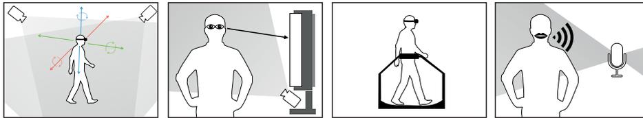
Figure 2.8: Non-hand input devices, from left to right: head and positional tracking, eye tracking, treadmill, and speech input.
