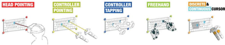
Figure 4.3: This figure illustrates our implemented selection-based text entry candidates for VR. From left to right: Head Pointing (HP, red), Controller Pointing (CP, yellow), Controller Tapping (CT, blue), Freehand (FH, green), Discrete (DC, orange) and Continuous Cursor (CC, light blue).
