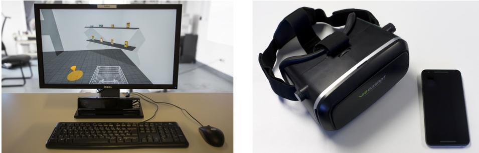
Figure 5.11: This figures show the **output devices** we used for our prototype. On the left: 22 inch display with Microsoft Kinect 2 for speech input and a standard mouse for camera control. On the right: a common smart-phone VR HMD and LG Nexus 5X.
